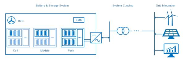
Figure 5. Schematic drawing of a battery storage system, power system coupling and grid interface components. Keywords highlight technically, and economically relevant aspects. Modified from [16].
