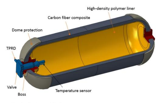
TPRD = Thermally Activated Pressure Relief Device
