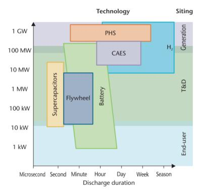
Figure 4: Electricity storage technologies [5]
