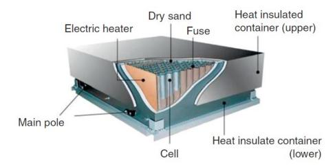
Figure 3: Illustration of Na-S battery module. [4]
