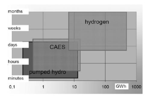
Figure 16: Timescale of storage technologies [61]
