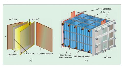
Figure 2: a) Reaction cell. b) Typical stack [2].
