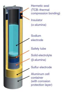
Figure 1: Schematic of a Na-S battery cell. [4]
