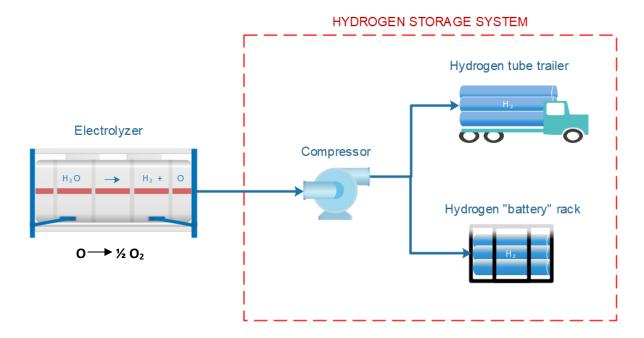
Figure 7: Typical pressurized tank storage system
