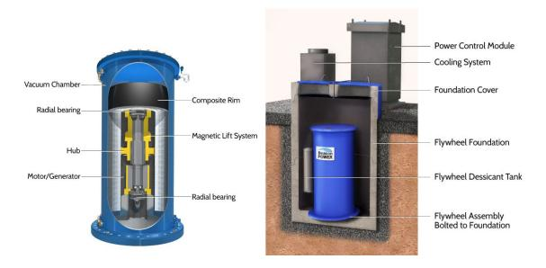
Figure 3: Drawing showing a cross section of the flywheel system and a visualization of how each module of a Beacon flywheel is mounted for operation [6]
