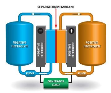
Figure 1: Schematic of flow battery [1].
