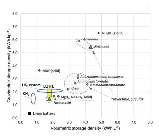
Figure 11: Properties of different hydrogen storage technologies [45]
