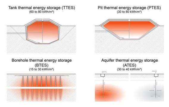
Figure 1: Seasonal thermal energy storage – concepts. Specific storage capacity given at typical operation temperatures of the given storage concepts [13].
