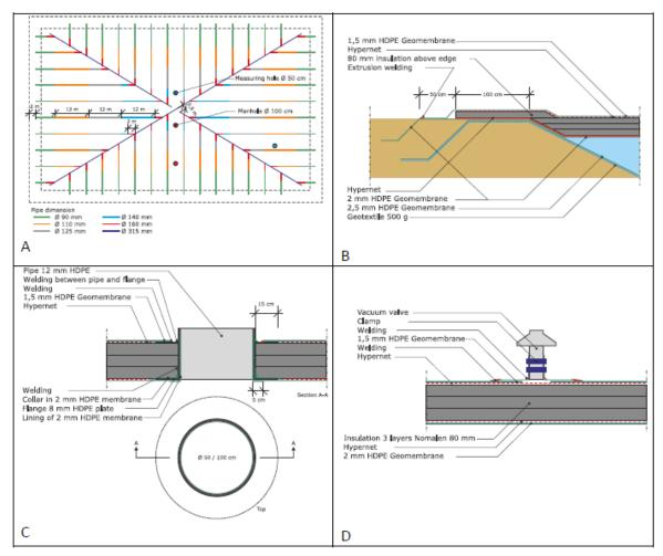
Figure 3: Illustrations of the lid in SUNSTORE 4 Marstal. A: the lid from above showing the pipes, B: the edge of the PTES, C: manhole, D: vacuum valve [1].
