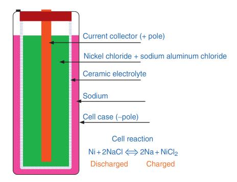
Figure 1: Schematic of Na-NiCl<sub>2</sub> battery cell. The "Ceramic electrolyte" is BASE [1].
