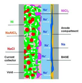
Figure 3: Illustration of Na-NiCl<sub>2</sub> charging process [2].
