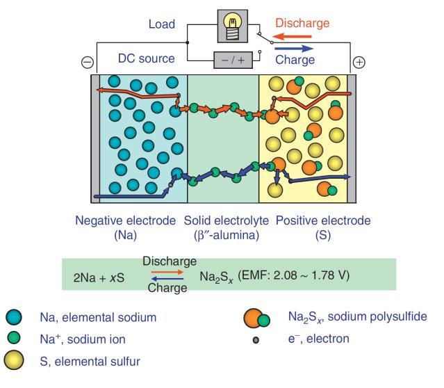
Figure 2: Graphical schematic of the reaction process and the full cell reaction. EMF: electromotive force. [4]
