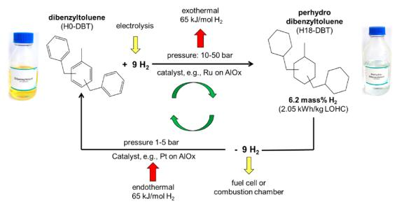
Figure 13: Hydrogen storage using DBT-LOHC system[50]
