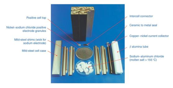
Figure 2: Na-NiCl₂ battery cell components [1].
