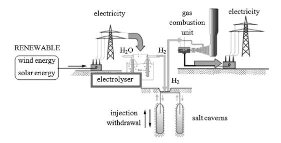
Figure 15: An illustration of H<sub>2</sub> storage in salt caverns. As an example it is shown that the hydrogen can be used for power generation. [56]
