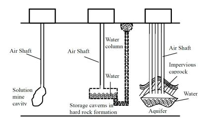
Figure 2: Various Geological Formations for Underground Storage [5]
