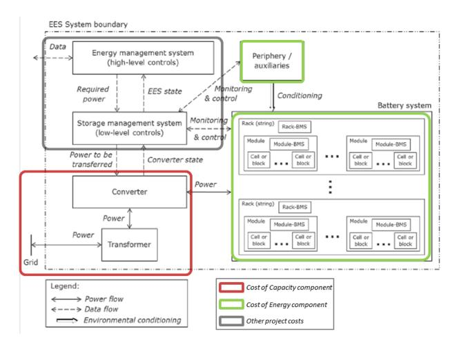
Figure 4 Components and their categorization for cell-based batteries, such as Li-ion, NaS and NaNiCl. Source: elaboration of [5].
