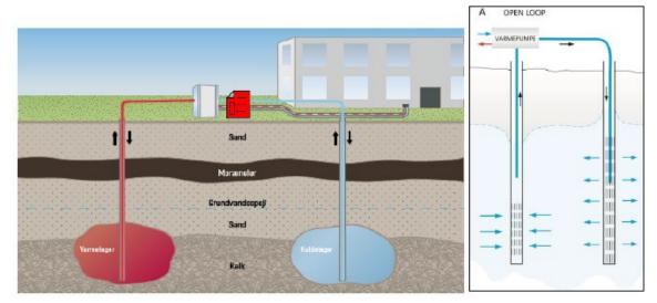
Figure 6: Principle of an ATES [1].
