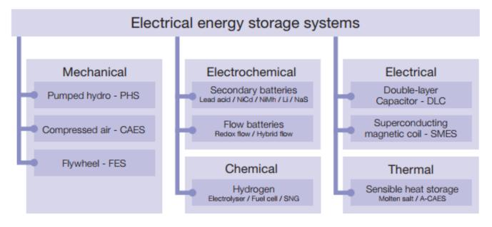
Figure 1 Classification of electrical energy storage systems according to energy form. Source [2]
