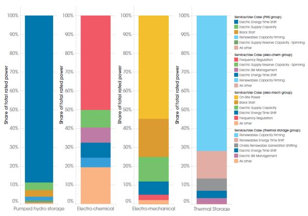
Figure 3 Global Energy Storage power capacity share by main use and technology group. Source [1].
