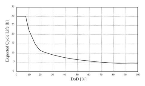
Figure 5: Expected number of cycles (in thousands) as function of Depth of Discharge (DoD) during cycles [9].
