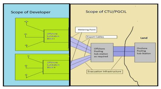
Figure 2.48 - Evacuation Infrastructure Network for Offshore Wind Farms
