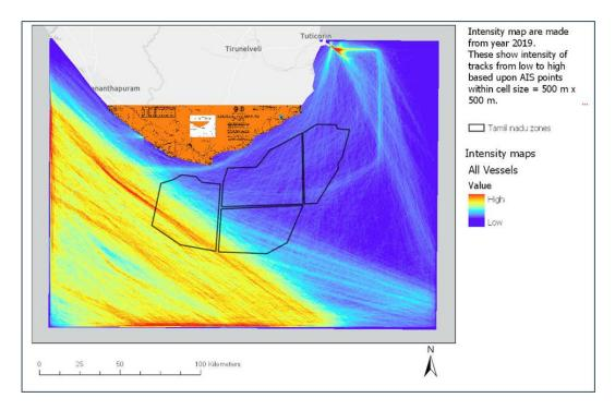
Figure 2.26 - Traffic intensity map around OWF zones – all vessels
