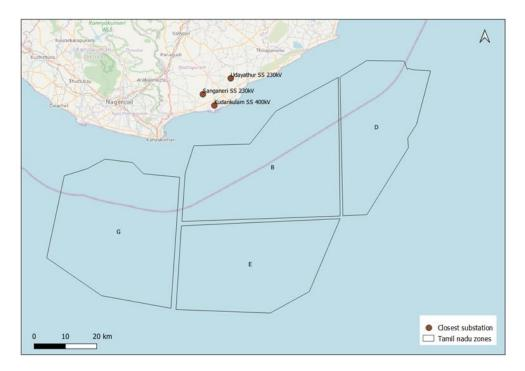
Figure 2.23 - Substations near the zone B (COWI, 2021)
