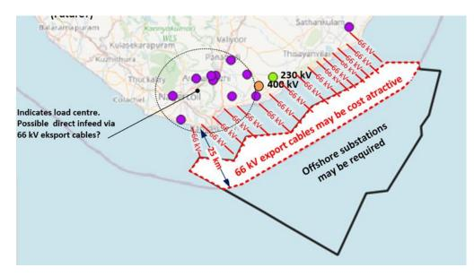
Figure 2.50 - Conceptual 66 KV connection to nearshore windfarms
