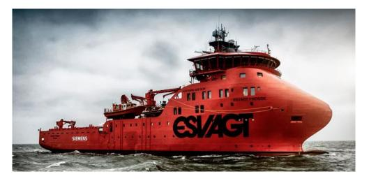
Figure 5-4 | Service Operation Vessel used by Siemens for servicing offshore wind farms (Esvagt, n.d.)
