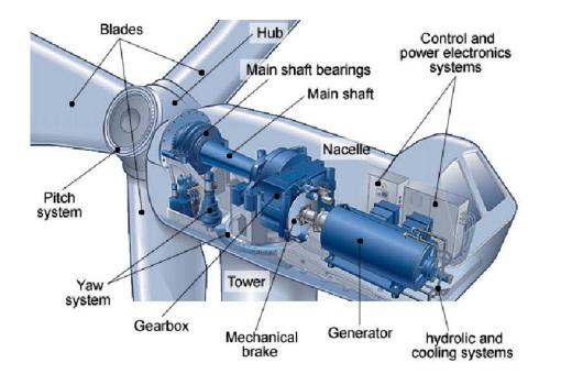
Figure 2-1 | Main components in an offshore wind turbine (Tchakoua, Wamkeue, & Theubou, 2013) in the concept/system sub-report)
