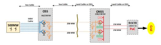
Figure 2.44 - High level topology for 500MW (with OSS)
