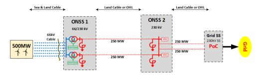
Figure 2.43 - High level topology for 500MW (without OSS)
