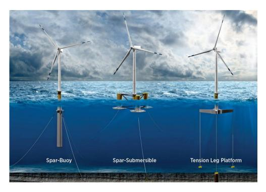
Figure 2-3| Visualization of different types of floating foundations (NREL, u.d.) in the concept/system subreport)
