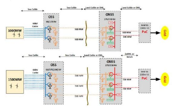
Figure 4.3 - typical 1 GW and 1.5 GW offshore wind farm electrical concept diagram (top: 1 GW, bottom:1.5 GW)
