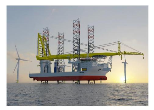
Figure 5-2 | Voltaire jack-up vessel (Jan De NUI Group)
