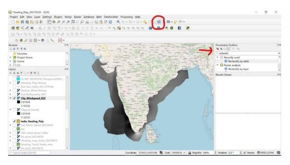
Figure 1.4: Clipped wind speed raster and processing toolbox
