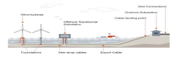
Figure 4.1 - Typical offshore wind farm infrastructure
