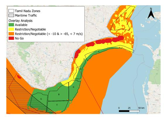
Figure 2.25 - Traffic light classification of offshore wind zones resulted from rough screening
