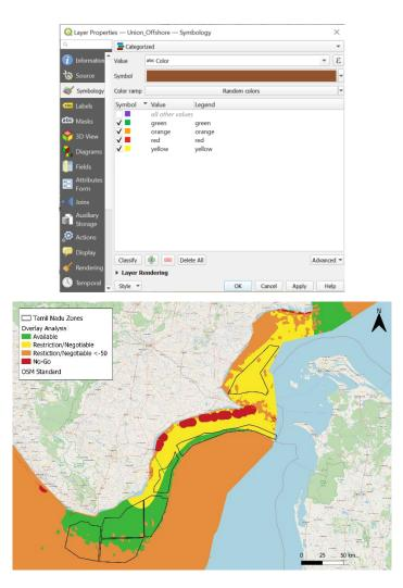
Figure 2.10: Layer properties window of the final output layer (left) and the color scheme applied on the final output layer
