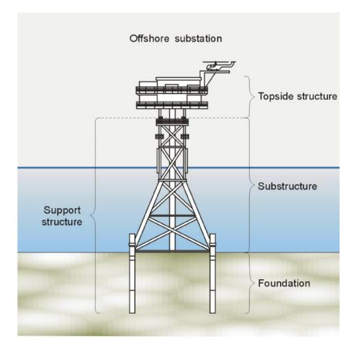
Figure 3-1 | A schematic of a typical offshore substation (Robak & Raczkowski, 2018) in the concept/system sub-report)
