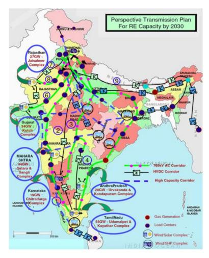
Figure 3.4 - Green energy corridor transmision plan by 2030
