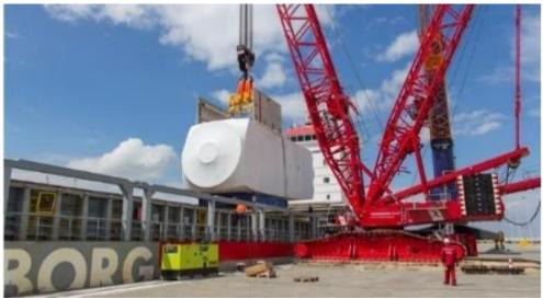
Figure 66: Figure Crawler cranes used in loadout of many major OWF components.
