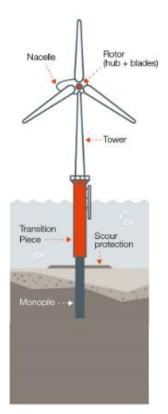
Figure 4: Components of a wind turbine
