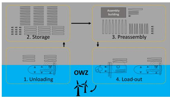
Figure 6: Diagrammatical layout for an installation port
