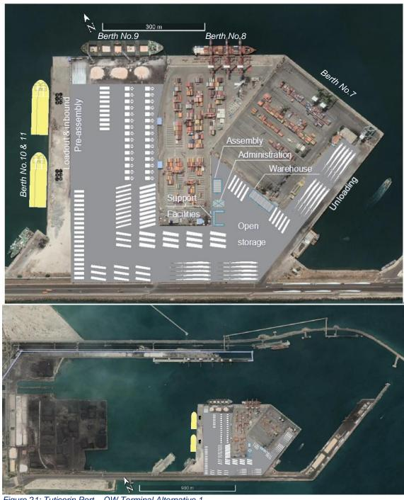
Figure 21: Tuticorin Port – OW Terminal Alternative 1
