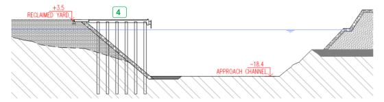
Figure 37: Vizhinjam port - Proposed sequence of works- 2
