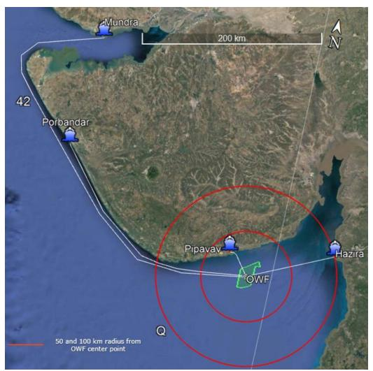
Figure 16: Candidates to support the installation of OWF along Gujarat coastline.
