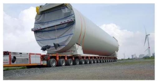
Figure 69: SPMT for transportation of large and heavy components
