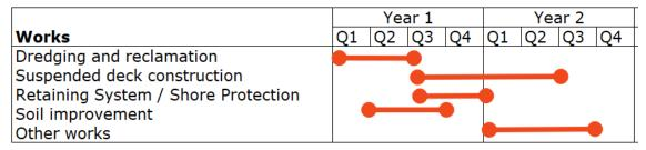
Figure 55: Pipavav Port – Indicative duration of works
