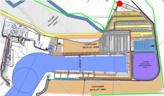
Figure 43: Hazira Port – Layout option for yards and berths to service OWF Shown within current port master plan layout
