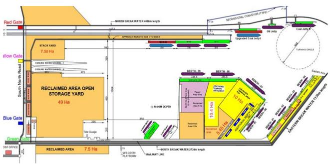
Figure 18: Tuticorin Port – Layout of existing harbour basin and terminals
