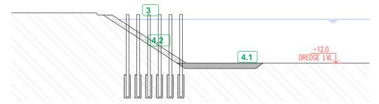
Figure 26: Tuticorin Port – Proposed sequence of works-2
