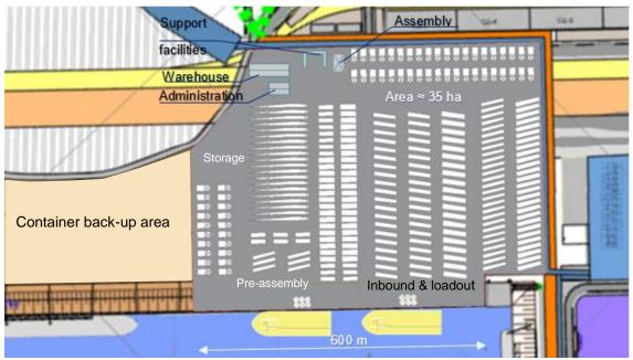
Figure 44: Hazira Port - Proposed port expansion for OWF
