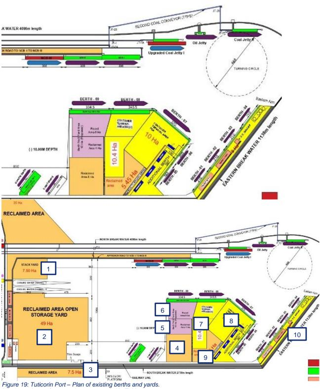
Figure 19: Tuticorin Port – Plan of existing berths and yards. Numbers given refer to yard areas as noted in Table 19.
