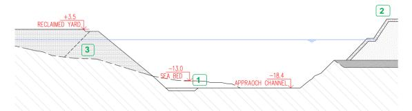
Figure 36: Vizhinjam port - Proposed sequence of works-1
