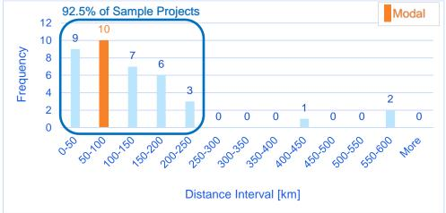
Figure 11: Distances between OWF and installation port facilities. (frequency in number of wind farms)
