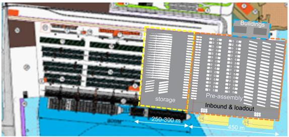
Figure 34: Vizhinjam Port – OW Terminal Alternative 3 Various options discussed for developing OW terminal. Orange dashed line represents exclusive OW Terminal. Yellow dashed line represents container terminal area used for temporary storage of lighter components.
