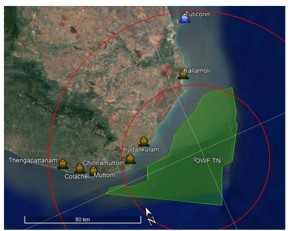
Figure 56: O&M Ports – Potential O&M bases for Tamil Nadu OWZ. Red curves denote 50km and 100km radius from OWZ central point.
