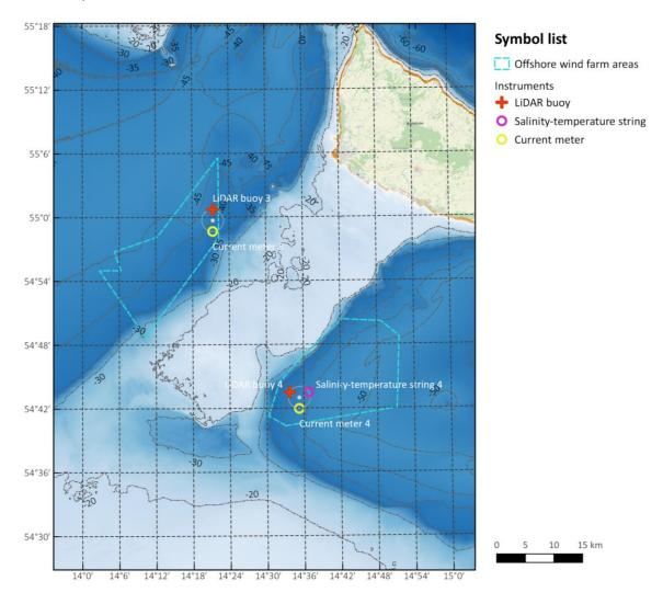
Figure 1-1 Instrument locations in the Energioe Bornholm project area
