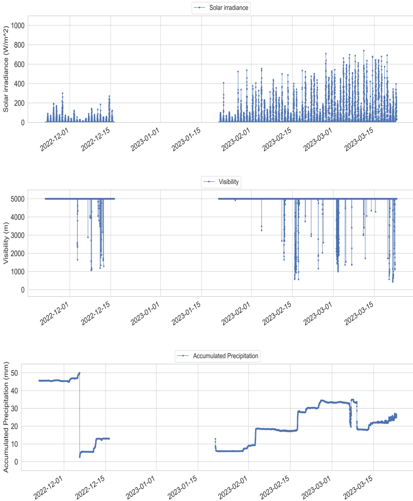
Figure B-16 Timeseries of air pressure, air humidity, air temperature, solar irradiance, visibility, and precipitation from November 2022 until March 2023. Please note that for precipitation, a jump from 50 mm to lower fill levels indicates emptying of the column when the maximum fill level is reached.
