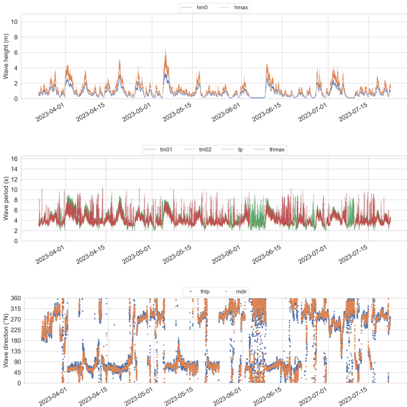
Figure B-11 Timeseries of wave heights, wave periods, and wave direction from March 2023 until July 2023. Please note that the y-axis for wave direction spans from 0° (bottom line) to 360° (top line).
