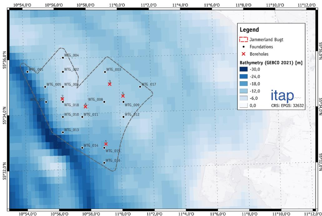
Figure 2: Possible Site layout of the OWF Jammerland Bay Near Shore Wind Farm according to alternative 1 with bathymetry (GEBCO 2021).
