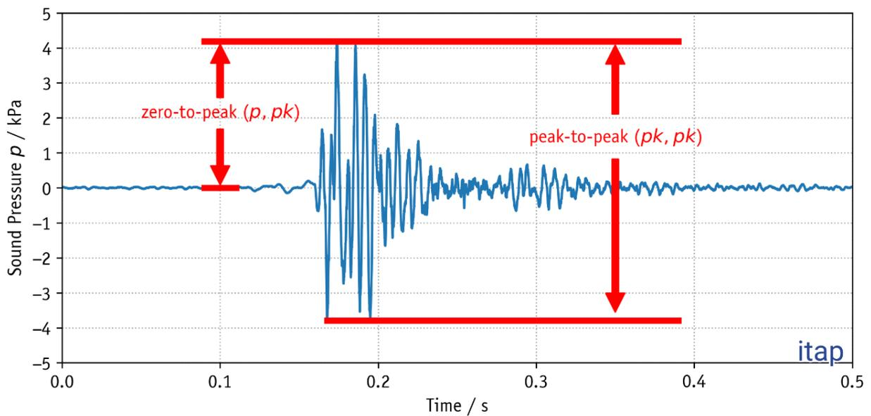
Figure 4: Typical measured time signal of underwater noise due to pile-driving in a distance of several 100 m.
