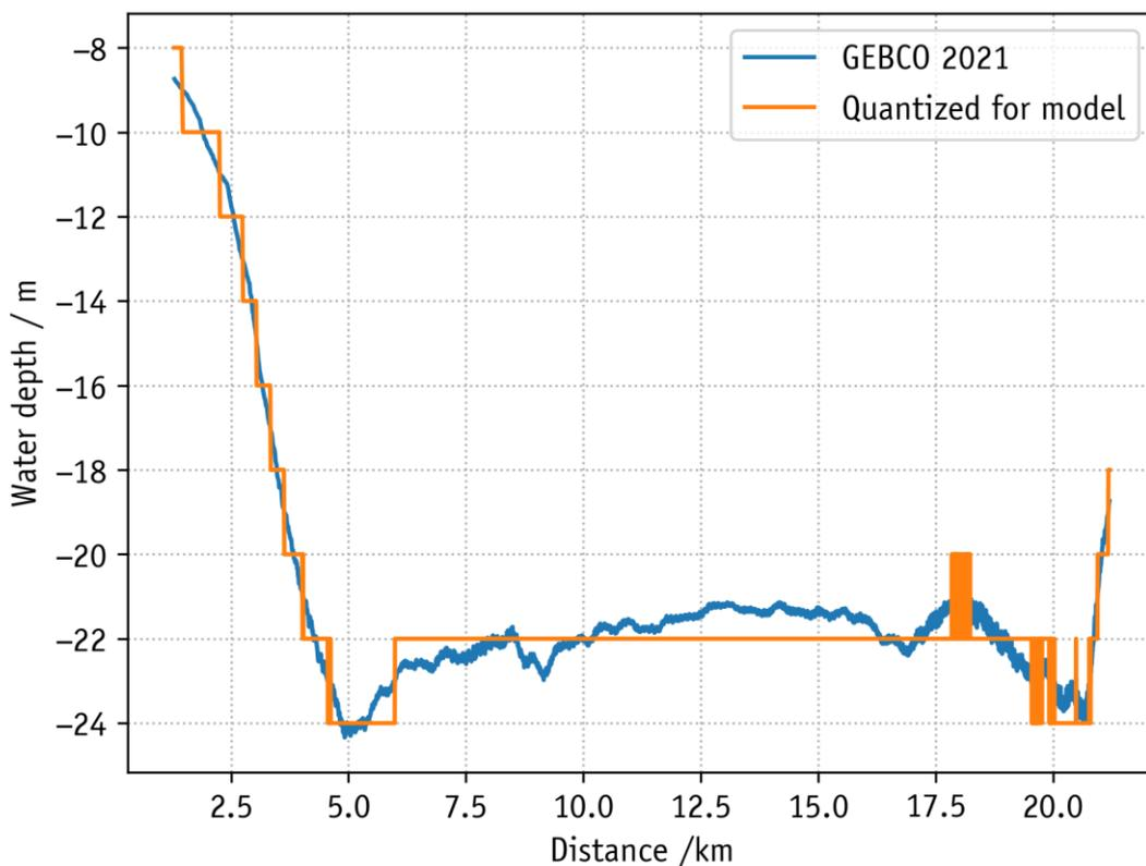
Figure 16: Waterdepth in 165° directions from WTG06 (preferred project design). Blue: Waterdepth according to GEBCO 2021 and orange: Quantized in 2 m steps used for modeling.
