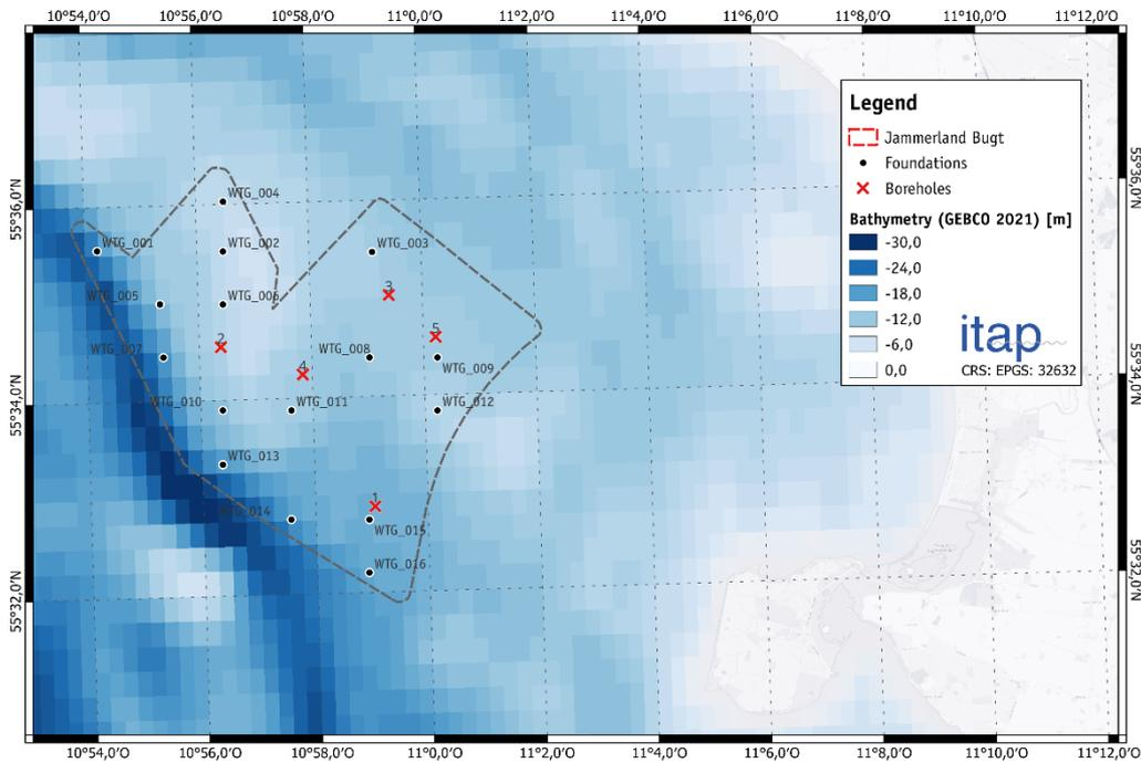
Figure 1: Possible Site layout of the OWF Jammerland Bay Near Shore Wind Farm according to the preferred project design with bathymetry (GEBCO 2021).
