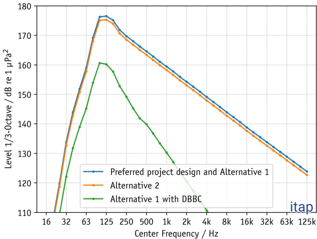
Figure 11: Reference Sound Exposure Level (SEL) in 1/3 octaves in 750 m distance for the considered locations in 9 m and 10 m water depth.
