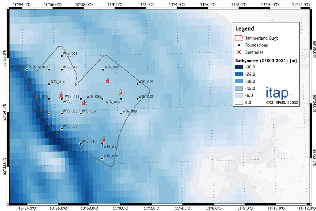
Figure 3: Possible Site layout of the OWF Jammerland Bay Near Shore Wind Farm according to alternative 2 with bathymetry (GEBCO 2021).
