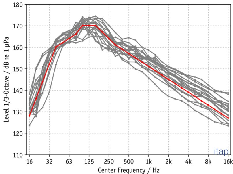
Figure 8: The model spectrum (red, blue) estimated for piling noise, based on different measuring data (grey: measuring data) for monopiles.
