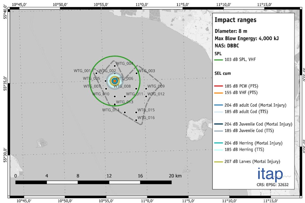
Figure 15: Impact ranges for during the installation of the 8.00 m monopile foundation at WTG6 (preferred project design) with a maximum blow energy of 4,000 kJ and a piling sequence of 3,424 blows. Top: without noise abatement system (unmitigated – no NAS). Bottom: mitigated with DBBC. The transmission loss estimated for 165° direction (Annex 1) used for all directions and water depths > 5 m.
