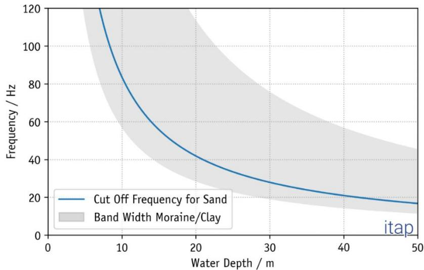
Figure 6: Theoretical, lower (limit) frequency ( $f_g$ ) for an undisturbed sound propagation in water as a function of the water depth for different soil stratifications (example adapted from (Urlick 1983) and (Jensen et al., 2010)); the example shows the possible range caused by different layers; the layer does not correspond to the layers in the construction field).
