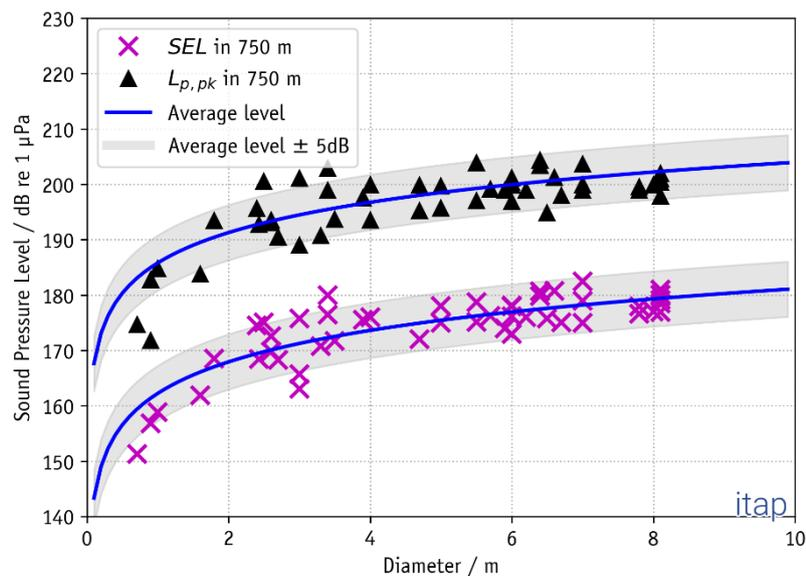
Figure 7: Measured zero-to-peak Sound Pressure Level ( $L_{p,pk}$ ) and broadband 5% exceedance Sound Exposure Levels ( $SEL_{05}$ ) at pile-driving construction works in 750 m distance at a number of OWFs as function of the pile diameter.
