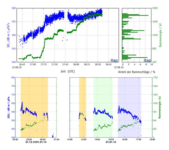
Figure 10: Top: Simple single event level (SEL) as a function of time (blue line) and the blow energy used (green line) for a typical monopile installation in the North Sea.
