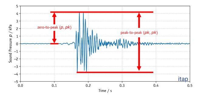
*Figure 4:* Typical measured time signal of underwater noise due to pile-driving in a distance of several 100 m.
