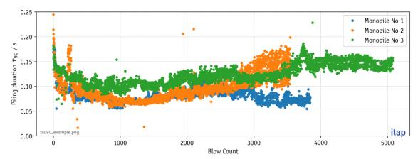
Figure 9: Pile-driving duration  $\tau_{90}$  of single strikes for three different monopile installations in accordance with de Jong et al. (2011).
