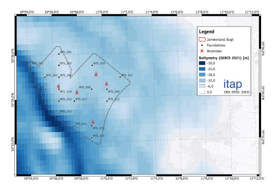
Figure 2: Possible Site layout of the OWF Jammerland Bay Near Shore Wind Farm according to alternative 1 with bathymetry (GEBCO 2021).
