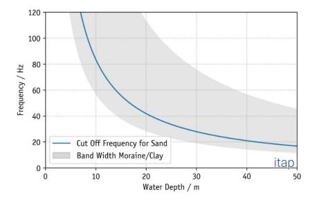
Figure 6: Theoretical, lower (limit) frequency  $(f_g)$  for an undisturbed sound propagation in water as a function of the water depth for different soil stratifications (example adapted from (Urick 1983) and (Jensen et al., 2010); the example shows the possible range caused by different layers; the layer does not correspond to the layers in the construction field).
