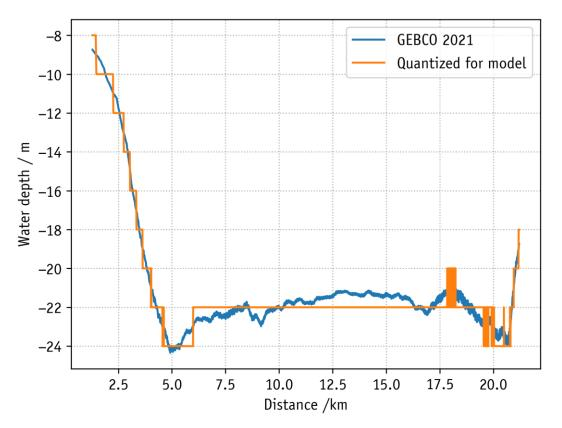
Figure 16: Waterdepth in 165° directions from WTG06 (preferred project design). Blue: Waterdepth according to GEBCO 2021 and orange: Quantized in 2 m steps used for modeling.
