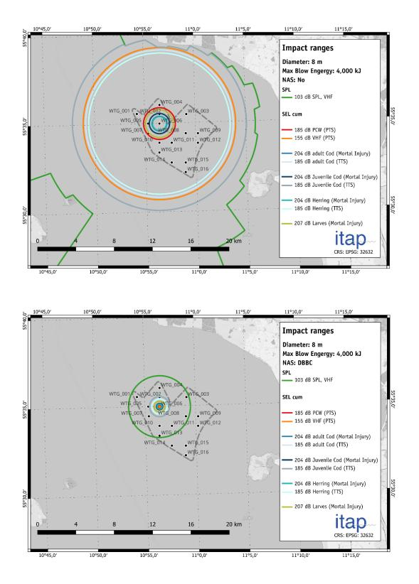
Figure 15: Impact ranges for during the installation of the 8.00 m monopile foundation at WTG6 (preferred project design) with a maximum blow energy of 4,000 kJ and a piling sequence of 3,424 blows. Top: without noise abatement system (unmitigated – no NAS). Bottom: mitigated with DBBC. The transmission loss estimated for 165° direction (Annex 1) used for all directions and water depths > 5 m.
