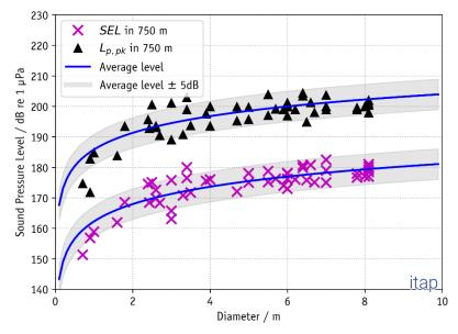
Figure 7: Measured zero-to-peak Sound Pressure Level  $(L_{p,pk})$  and broadband 5 % exceedance Sound Exposure Levels (SEL<sub>05</sub>) at pile-driving construction works in 750 m distance at a number of OWFs as function of the pile diameter.
