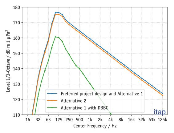
Figure 11: Reference Sound Exposure Level (SEL) in 1/3 octaves in 750 m distance for the considered locations in 9 m and 10 m water depth.
