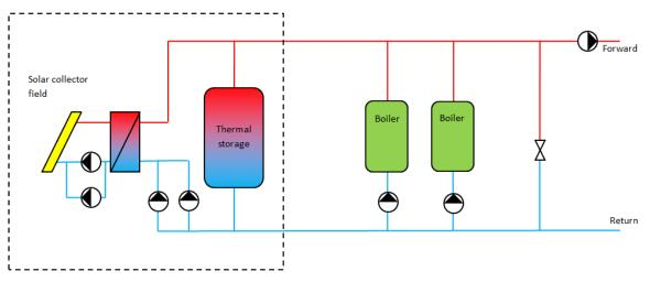
Figure 4 Schematic drawing of a possible system integration of solar district heating [5].
