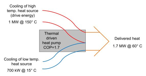
Figure 5 The high temperature drive energy of 1 MW enables the heat pump to utilize 700 kW from a low temperature heat source at 15 °C. Thus delivering 1.7 MW at 60 °C (COP is 1.7).
