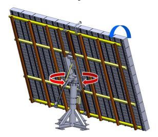
Figure 5 A generic dual axis PV system (Ref. 11)
