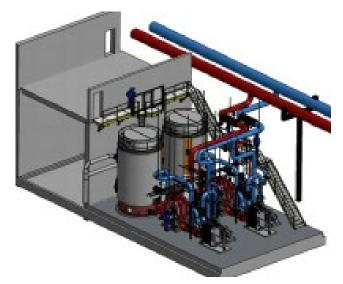
Figure 2: Illustration of 2x40 MW electric boilers installed at Studstrup power plant. The heat exchangers in front of the electric boilers transfer the heat from the water circuit in the boiler to the district heating circuit (blue/red piping). [9]
