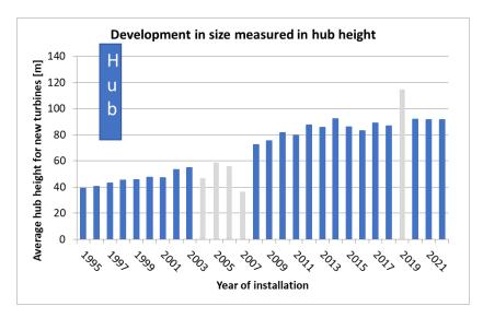
Figure 19 Average hub height for new turbines (rated power > 25 kW) [2]
