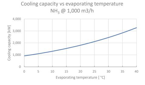
Figure 4 Cooling capacity of a specific compressor dependent on evaporating temperature.
