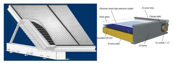
Figure 1 Basic principle of a flat plate solar collector
