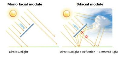
Figure 3 Bifacial module structure (Ref. 12).
