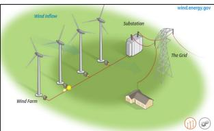
Figure 11 General turbine technology and electrical system.
