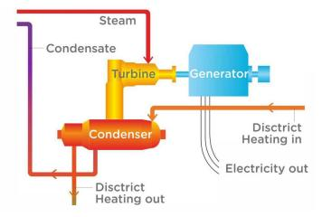
Figure 3 Turbine/generator system of backpressure CHP
