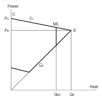
With the steam boiler at full capacity, the turbine may be operated at all points along the line C-B. In the real world, C-B may not be a straight line, but a linear relationship is a good proxy.
