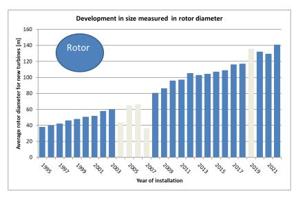
Figure 18 Average rotor diameter for new turbines (rated power > 25 kW) [2]
