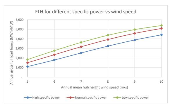
Figure 16 Annual full load hours as a function of mean wind speed at hub height. The examples in the figure are 3 MW with 90m rotor diameter, specific powers are 472 W/m2 called "high specific power" and 3.3 MW turbines with 112 m and 126 m rotor diameters, specific powers are 335 W/m² called "medium specific power" and 265 W/m² called "low specific power".
