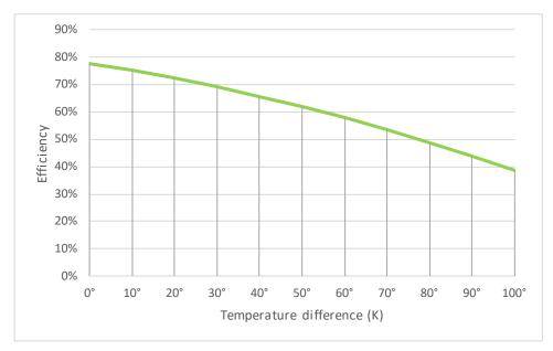
Figure 3 Efficiency as a function of temperature difference. (Based on data from [8], example with G=1.000 W/m²,  $\eta_0$ =0.777,  $a_1$ =2.41,  $a_2$ =0.015)<sup>23</sup>
