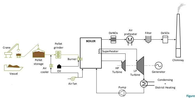
1: Sketch of a CHP plant converted to firing with wood pellets. The green elements indicate the equipment that needs to be added, replaced or refurbished.
