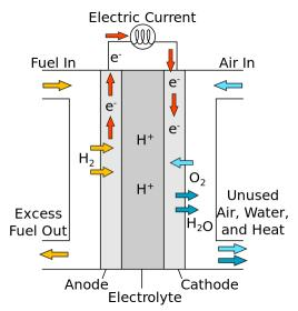
Figure 1: Diagram of a PEM-FC [2].
