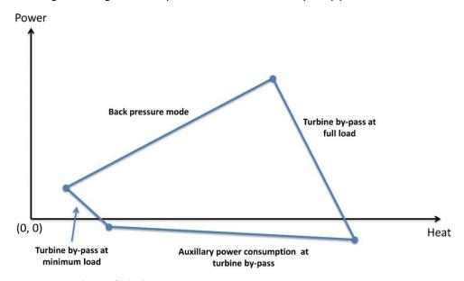
Figure 4 Generic PQ-diagram for backpressure CHP
