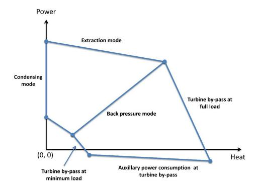
Figure 5 Generic PQ-diagram for extraction CHP
