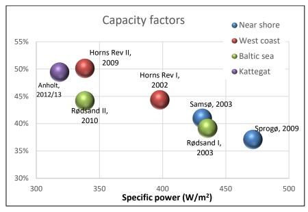
Figure 7 Capacity Factor shown as function of the Specific Power (W/m2) for Danish Offshore wind turbine projects. The three projects most left are the latest ones among the sample. (Figure from previous version of Technology Catalogue, not updated from table above).
