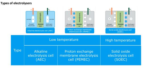
Figure 4 The three primary electrolyser technologies: AEC, PEMEC, and SOEC.
