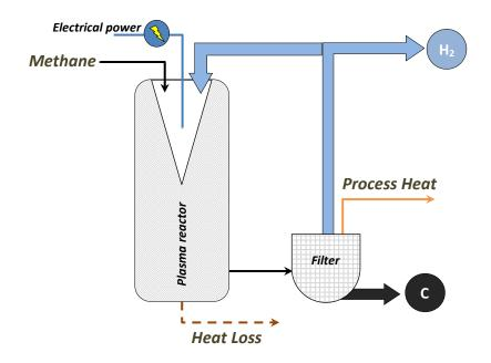
Figure 4. Plasma-assisted Decomposition Diagram.
