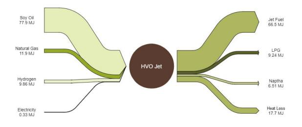
Figure 2 HVO Jet Fuel Energy Balance
