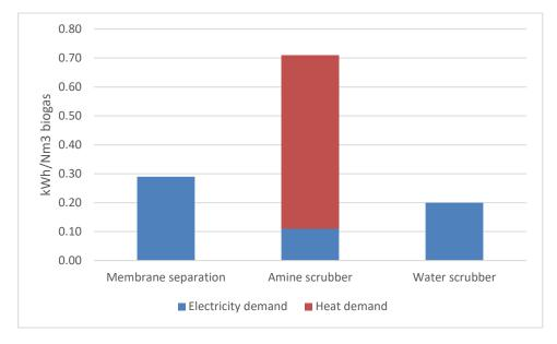
Figure 12: Energy consumption (kWh/Nm<sup>3</sup> raw biogas) for the upgrading technologies, water scrubbing, amine scrubber and membrane
