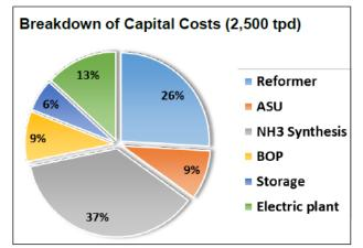
Figure 15. Cost split on main systems in a conventional NH<sub>3</sub> plant from Linde [10]. Reformer, electric plant (power plant) and some balance of plants (BOP) will disappear for a green NH<sub>3</sub> plant. Cost of green NH<sub>3</sub> plant (excl. electrolysis unit and ASU) is therefore taken as 54% of conventional plant, based on all obtained data.
