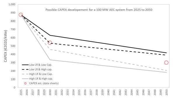
Figure 13 Possible CAPEX development for a 100 MW AEC system from 2025 to 2050.
