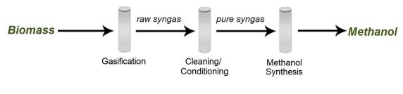
The overall process is shown in the following simplified process flow diagram.
