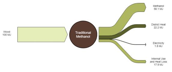
Figure 3 GreenSynFuels Traditional Methanol Plant
