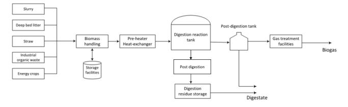
Figure 6: Typical components in a biogas plant. OBS alternative terms for technical description might be used by some actors: e.g., biomass handling might be referred to as pre-treatment, digestion reaction tank as a digester and digestion residue storage as digestate storage or post-storage of digestate.
