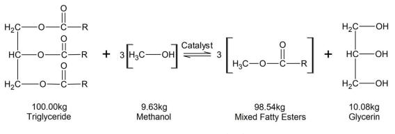
**Figure 4 Basic Biodiesel Reactions**
