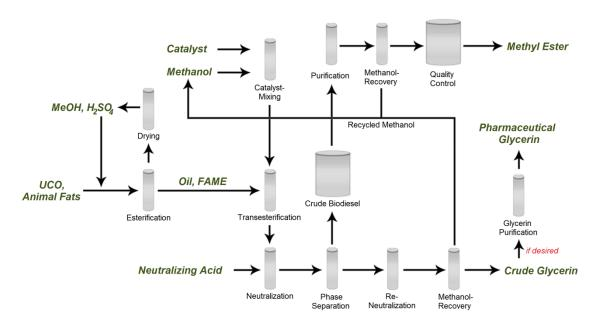
Figure 1 Two Step Biodiesel Production Process
