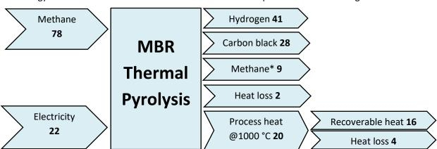
The energy balance for MBR thermal-assisted methane decomposition is shown in Figure 6.
