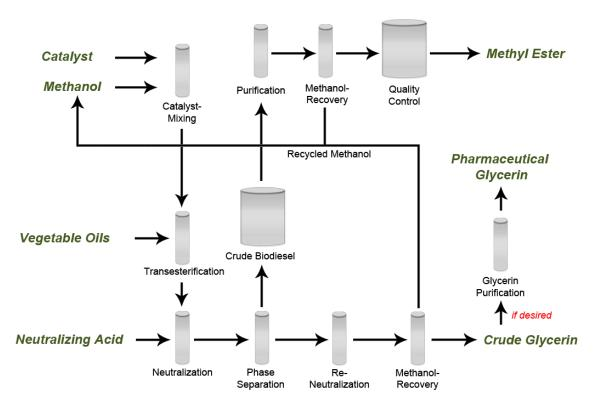
Figure 1 Biodiesel Production Process
