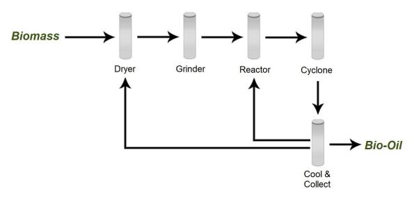
Figure 1 Fast Pyrolysis Process Flow
