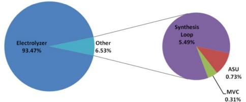
Figure 13: Power requirement breakdown for a green ammonia plant (MVC=Mechanical Vapor Compression, includes pumping and desalination of feed water to electrolysis unit) [ref 7].
