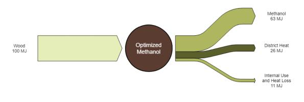
**Figure 4 Optimized Biomass to Methanol Plant**
