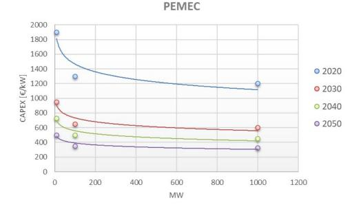
Figure 15 CAPEX of electrolyser plant, based on scale and time for PEMEC.
