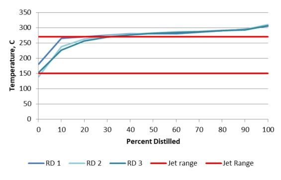
Figure 5 Renewable Diesel Distillation Curves
