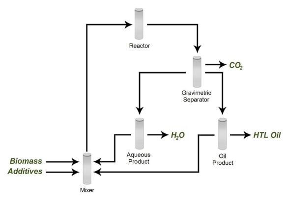
Figure 1 Hydrothermal Liquefaction Process Flow
