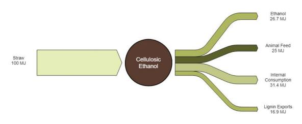
Figure 4 Inbicon Cellulosic Ethanol Energy Balance
