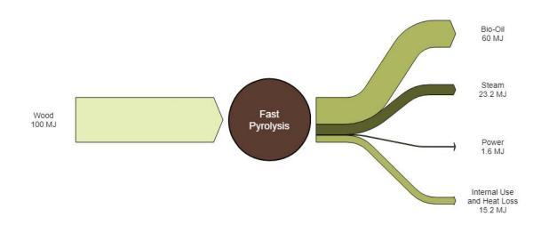
Figure 2 Fast Pyrolysis Oil Energy Balance
