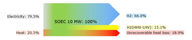
Figure 11 The energy inputs and outputs of an SOEC (2020, 10 MW hydrogen plants). Data is derived from Ramboll references.
