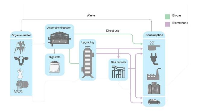
Figure 10: Biogas may either be used directly as an energy source or be upgraded through an upgrading plant to be fed into the gas network or be directly applied for consumption needing gas with high energy content. Illustration from IEA [2]
