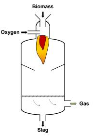
Principle of the entrained flow gasifier.
