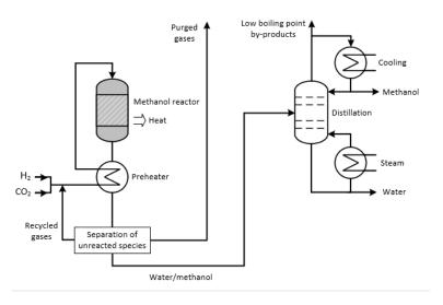
Figure 2: Simplified sketch of a hydrogen to methanol production plant.
