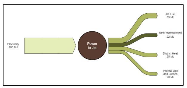
Figure 2: Power to Jet Fuel Energy Balance 2050 Projection
