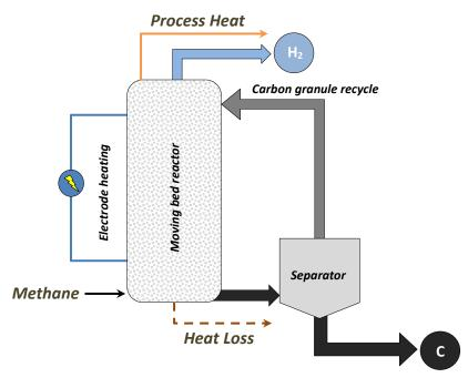
Figure 3. Thermal-assisted (moving-bed reactor) Decomposition Diagram.
