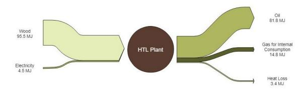
Figure 2 Hydrothermal Liquefaction Energy Balance
