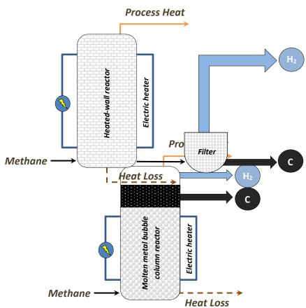
Figure 1. Thermal-assisted (heated-wall) Decomposition Diagram.
