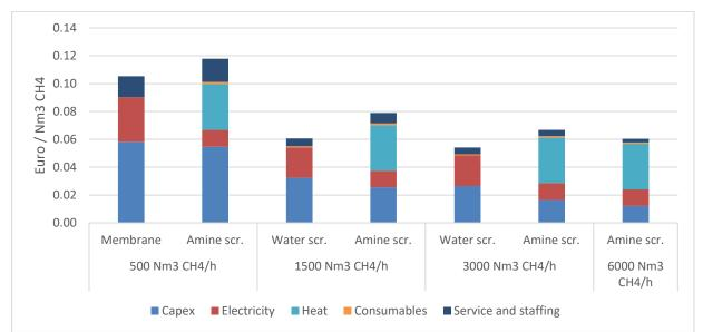
The cost figures include regenerative thermal oxidation (RTO) to treat the methane loss of around 1% at the water scrubbing plants, however, the value of the loss of biogas is not considered in the comparison.
