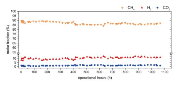
Figure 5 Gas Composition Prior to Final Clean-up
