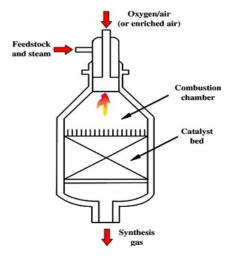
Figure 5: Autothermal reformer (ATR)
