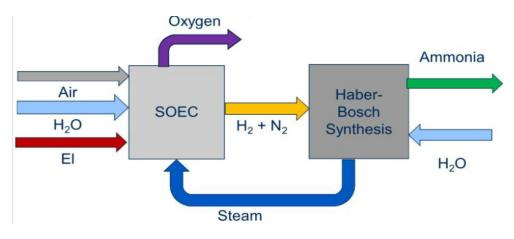
Figure 11: SOC4NH3 project combining electrolysis unit and ASU (El = power)[ref 15]
