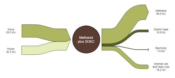
**Figure 5 Hybrid Biomass to Methanol Plant**
