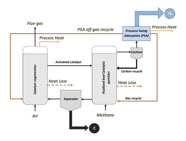
Figure 5. Fluidized Bed Catalytic-assisted Decomposition Diagram.
