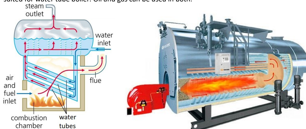
Figure 1: Schematic of a furnace producing steam or hot water. (Left) is a water tube boiler and (Right) is fire tube boiler.
