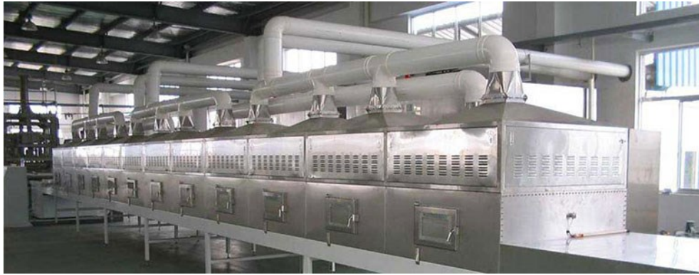
Figure 3. Industrial microwave heating system (Max Industrial Microwave)
