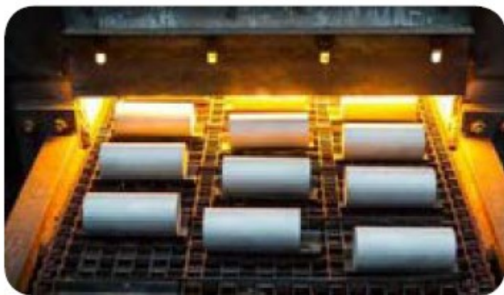
Figure 4: Queen City Forging - heating billets, from [1]
