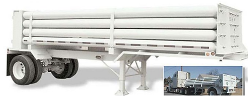
Figure 22: Trailer and storage is same vessel.
