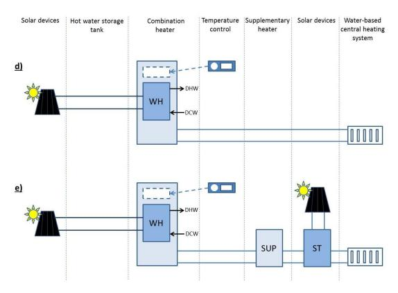
Figure 2 Examples of packages containing combination heaters
