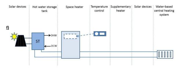
Figure 3 Example of package containing space heaters, where the solar devices are not part of the package
