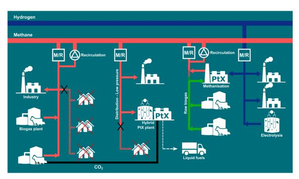
Figure 21: How the future gas system in Denmark may develop into multiple parallel systems. Source: Danish Energy Agency
