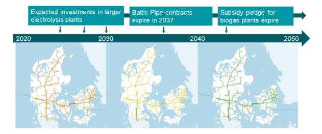
Figure 19: The map illustrates conversion possibilities in the existing gas system in the period 2020-2050. Note 1: Orange: Agreement restricts use of the gas system to a specific purpose. Yellow: Agreement restricts use of the gas system to a specific purpose, but some sections may allow other uses. Green: The gas system can be used for other purposes.
