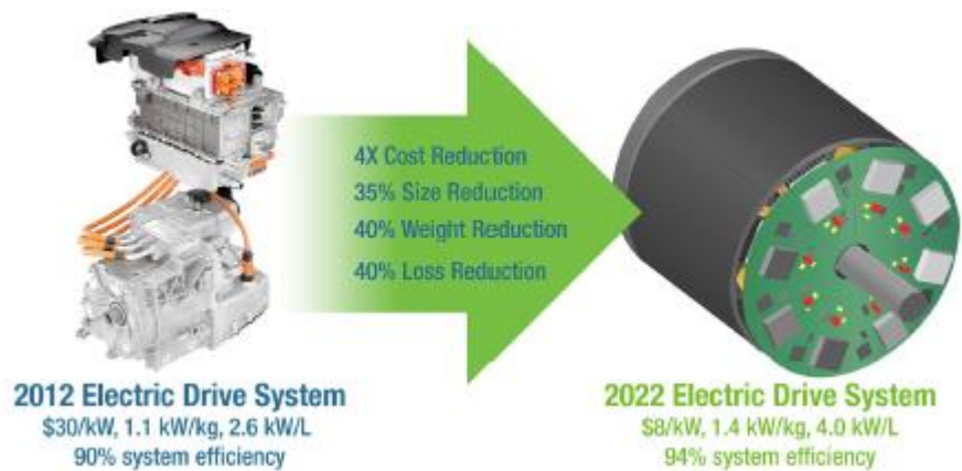
Figure 12: Electric drive system advancement targets in the DOE's EV Everywhere Grand Challenge Blueprint (US Department of Energy, 2013a).
