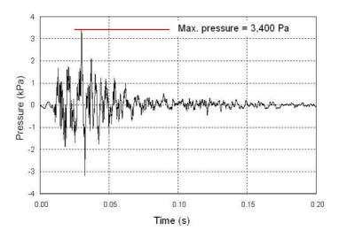
Figure 3.14. Waveform of a impact-pile pulse (after ITAP, 2005).
