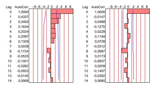
Figure 3.9. Time series of daily click frequencies and the residual series from a station 7 deployment in 2005. The autocorrelation graph is shown below, indicating lag 1 and lag 2 autocorrelation (left graph) for the transformed frequencies and no autocorrelation in the residuals (right graph).
