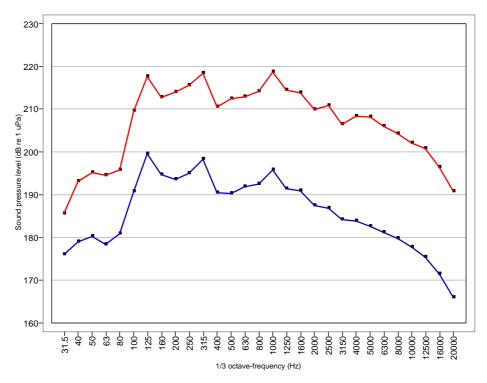
Figure 3.15. Frequency spectrum (Third octave band sound pressure level) of ramming pulses (FINO 1platform) back-calculated to 1 m (red =  $dB_{0-p}$  re 1  $\mu$ Pa, blue =  $dB_E$  re 1  $\mu$ Pa from ITAP, 2005).
