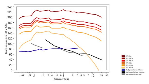
Figure 6.2. Pile-driving noise and background noise (see Figure. 6) compared to the audiogram of harbour porpoises and harbour seals (audiogram values as dB<sub>rms</sub> re 1 μPa; after Kastelein et al., 2002 and Kastak & Schusterman, 1998).
