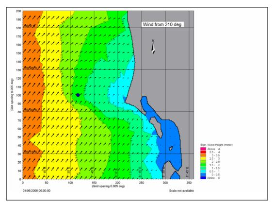
Figure 4.4 Wave pattern over Horns Rev area for constant wind speed of 15 m/s for wind direction 210°.
