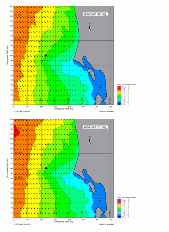
*Figure 4.1* Wave patterns over Horns Rev area for constant wind speed of 15 m/s for wind directions 330° and 310°.
