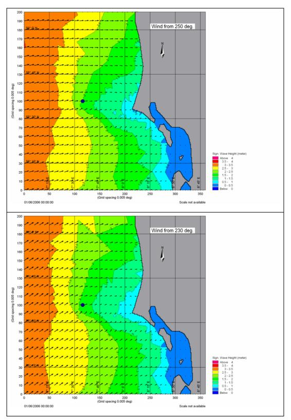
*Figure 4.3* Wave patterns over Horns Rev area for constant wind speed of 15 m/s for wind directions 250° and 230°.
