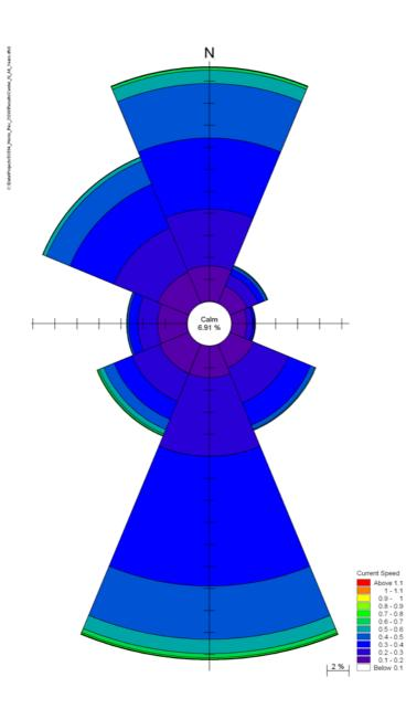
*Figure 5.3 Directional distribution of current speeds in the Central Point (55.60 N; 7.58 E). For location, see Figure 4.5.*
