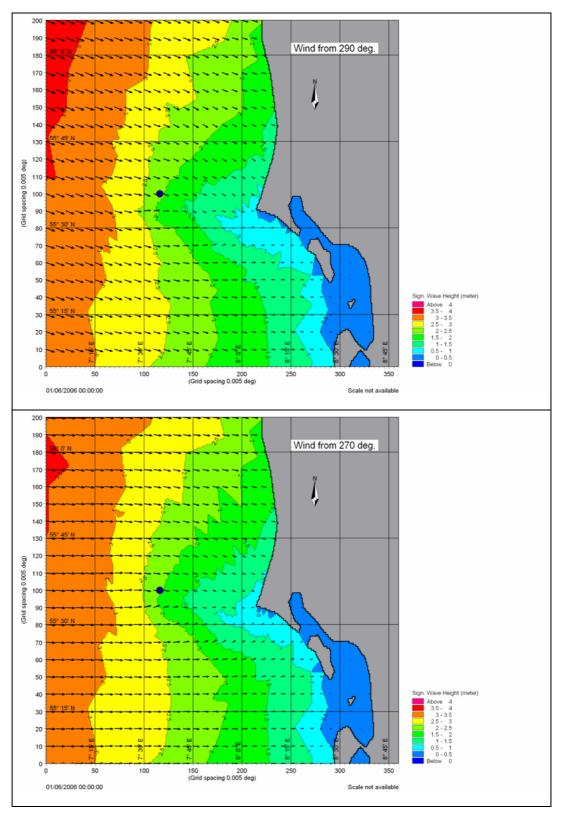
*Figure 4.2* Wave patterns over Horns Rev area for constant wind speed of 15 m/s for wind directions 290° and 270°.
