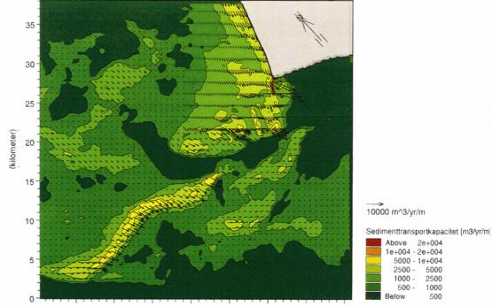
Figure 3.7 Transport conditions for the February 1999 storm, which was dominated by waves from WNW to NW, Ref. /4/.
