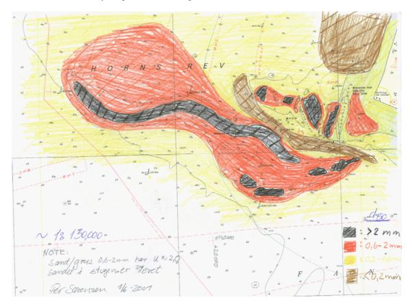
Figure 3.6 Distribution of mean grain diameter at Horns Rev, from Ref. /4/.
