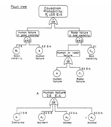
Figure 7-1: Fault tree for causation (human failure) probability.
