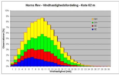
Figure 3-2: Distribution for the wind velocity.
