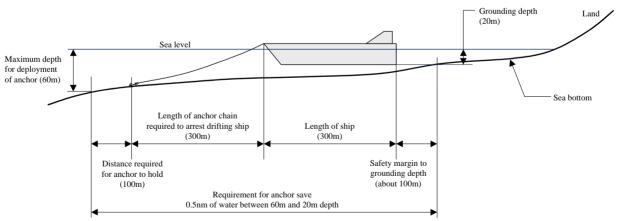
Figure 13-8: Graphical representation of the Anchor save mechanism
