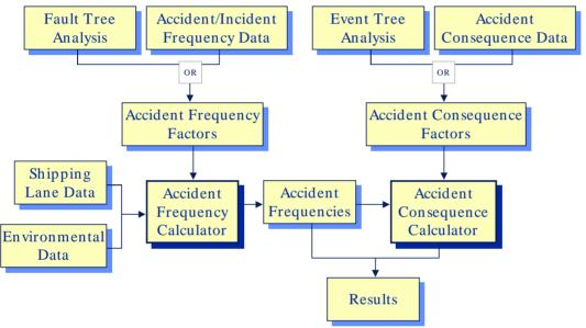
Figure 13-1: Block Diagram of MARCS
