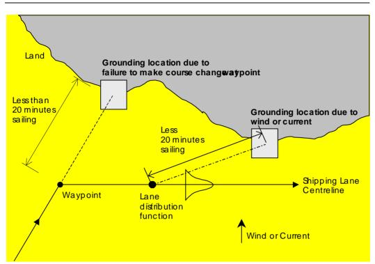
Figure 13-5: Graphical representation of the powered grounding model
