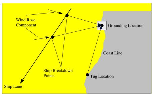
Figure 13-6: Graphical representation of the drift grounding model
