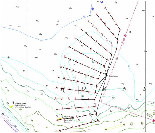
Figure 4-2: Wind turbine configuration for the "Nord" location.
