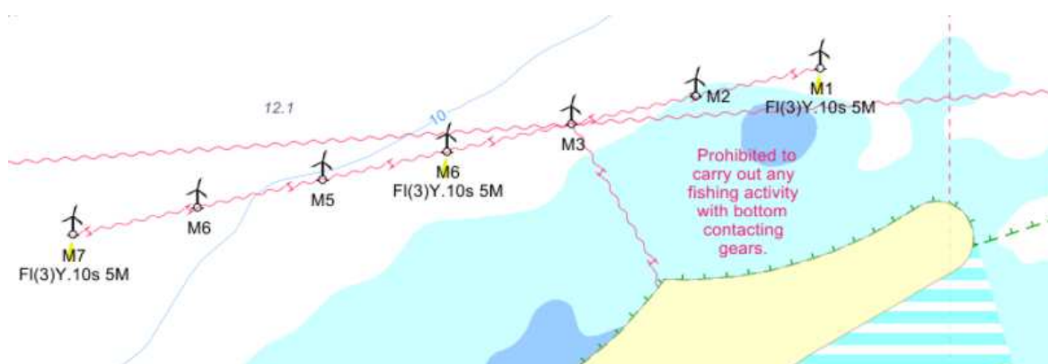
Figure 3-5 Example charting of offshore wind farm where three of the turbine have light flashing synchronously. All turbines are marked with ID, and the power cable grid is also shown in the chart.
