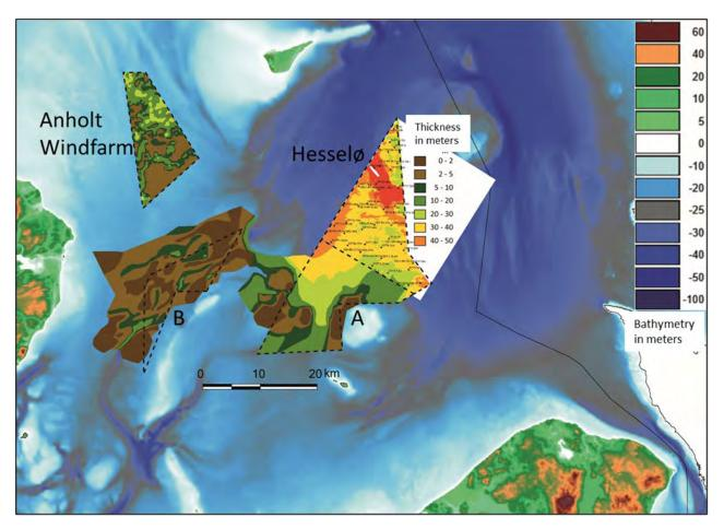
Figure 1.1 Thickness of geotechnical soft sediments in the southern Kattegat Anholt OWF and potential Hesselø, Area A and B. For details see Appendix C.
