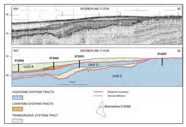
Figure 6.2. Boomer seismic section 572008.
