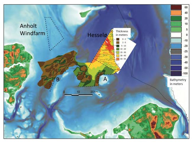
Figure 10.6 General thickness of geotechnical soft sediments (combined thickness of Unit A–E/F Seismic data) in Area A and B, compared to the detailed mapping of Hesselø OWF.
