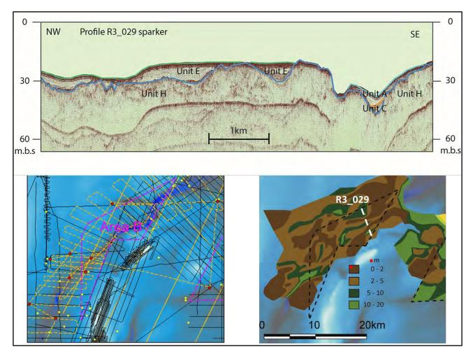
Figure 10.2 North-west to south-east Sparker line R3\_035 with documentation for location in relation to the seismic archive data grid (black lines are sparker lines) and the geotechnical soft sediment thickness map.
