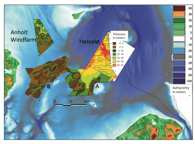
Figure 13.1 Thickness of geotechnical soft sediments in the southern Kattegat Anholt OWF and potential Hesselø, Area A and B. For details see Appendix C.
