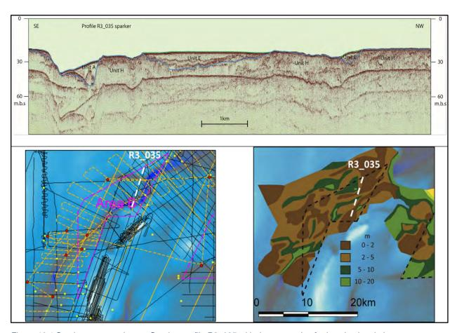
Figure 10.1 South-east to north-west Sparker profile R3\_035 with documentation for location in relation to the seismic archive data grid and the geotechnical soft sediment thickness map.
