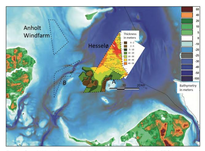
Figure 9.4 General thickness of geotechnical soft sediments (combined thickness of Unit A–E/F Seismic data) in Area A compared with the detailed mapping of Hesselø OWF.
