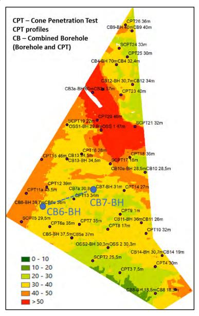
Figure 7.3 Thickness of geotechnical soft sediments (thickness of Unit A–E/F Seismic data) in the Hesselø OWF. Point data shows thickness of soft sediment (CPT and boreholes). There is generally a good correlation between the data sets. Local areas without correlation could be related to glacial disturbance of Unit E/(F). Figure from Energinet (2021).
