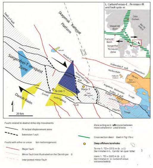
Figure 5.1. Regional structures in the southern part of the Kattegat (Erlström and Sivhed 2001). The locations of the existing Anholt OWF (light blue), the planed Hesselø OWF (dark blue) as well as the potential OWF areas A and B (yellow) are indicated.
