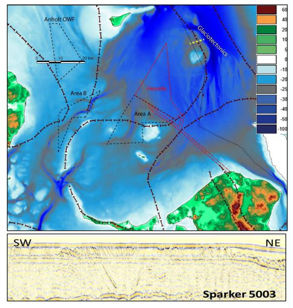
Figure 5.6. Upper figure: Interpreted ice marginal ridges in the southern part of the Kattegat. Lower figure: Sparker profiler showing evidence of glaciotectonic deformations north of Store Middelgrund (yellow dashed line on upper figure). Bathymetry from Emodnet. The location of the OWF's is indicated.
