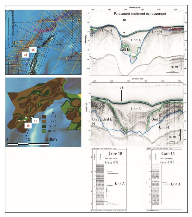
Figure 10.5 Parasound echosounder profiles from the southernmost part of Area B, with documentation for locations in relation to the seismic archive data grid (yellow lines are parasound grid). The positions of the seismic profiles and vibrocores 18 and 15 are indicated on the geotechnical soft sediment thickness map. Core descriptions with indication of seismic units.
