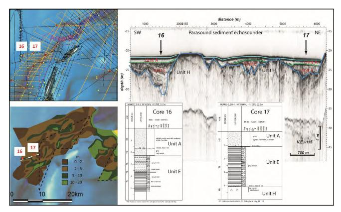
Figure 10.4 Parasound echosounder lines west of Area B, with documentation for location in relation to the seismic archive data grid (the yellow lines show the parasound grid). The positions of the seismic examples and vibrocores 16 and 17 are indicated on the geotechnical soft sediment thickness map. Core descriptions with indication of seismic units.
