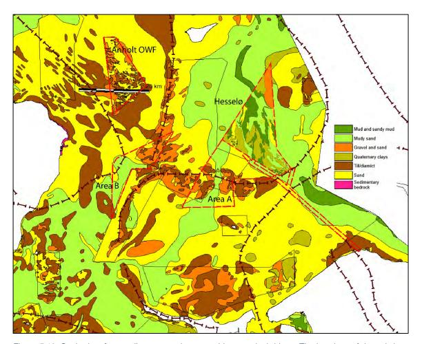
Figure 5.10. Seabed surface sediment map, interpreted ice marginal ridges. The locations of the existing Anholt OWF, the planed Hesselø OWF and the potential OWF areas A and B in the southern part of the Kattegat are indicated (red stippled polygons). Updated detailed sediment data from Fugro (2021) is presented in Hesselø OWF. (Black lined polygons marks margins of detailed mapped subareas).
