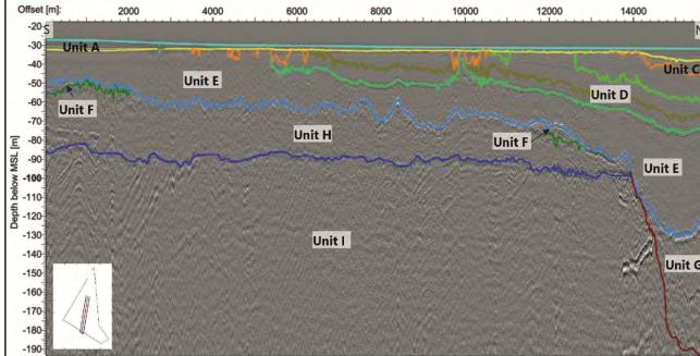
Figure 6.1. Overview of seismostratigraphic units interpreted in the Hesselø OWF study area.
