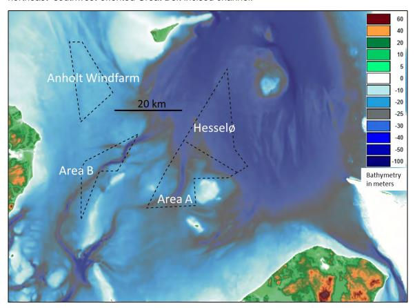
Figure 5.9 Southern Kattegat bathymetry. The locations of the existing Anholt OWF, the planed Hesselø OWF and the potential OWF areas A and B in the southern part of the Kattegat are indicated. Bathymetry from www.emodnet-bathymetry.eu.
