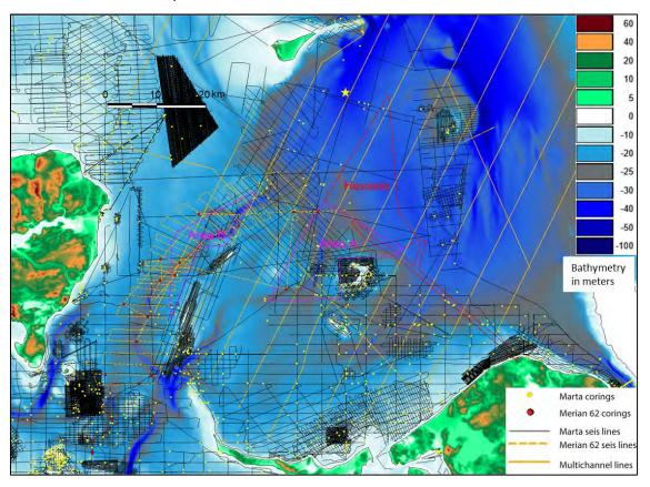
Figure 4.1. Distribution of Marta database seismic grid and core data in the southern and central Kattegat region. The planed Hesselø OWF and cable transects (red polygons) as well as the potential OWF areas A and B (purple polygons) the southern part of the Kattegat region. Bathymetry from www.emodnet-bathymetry.eu
