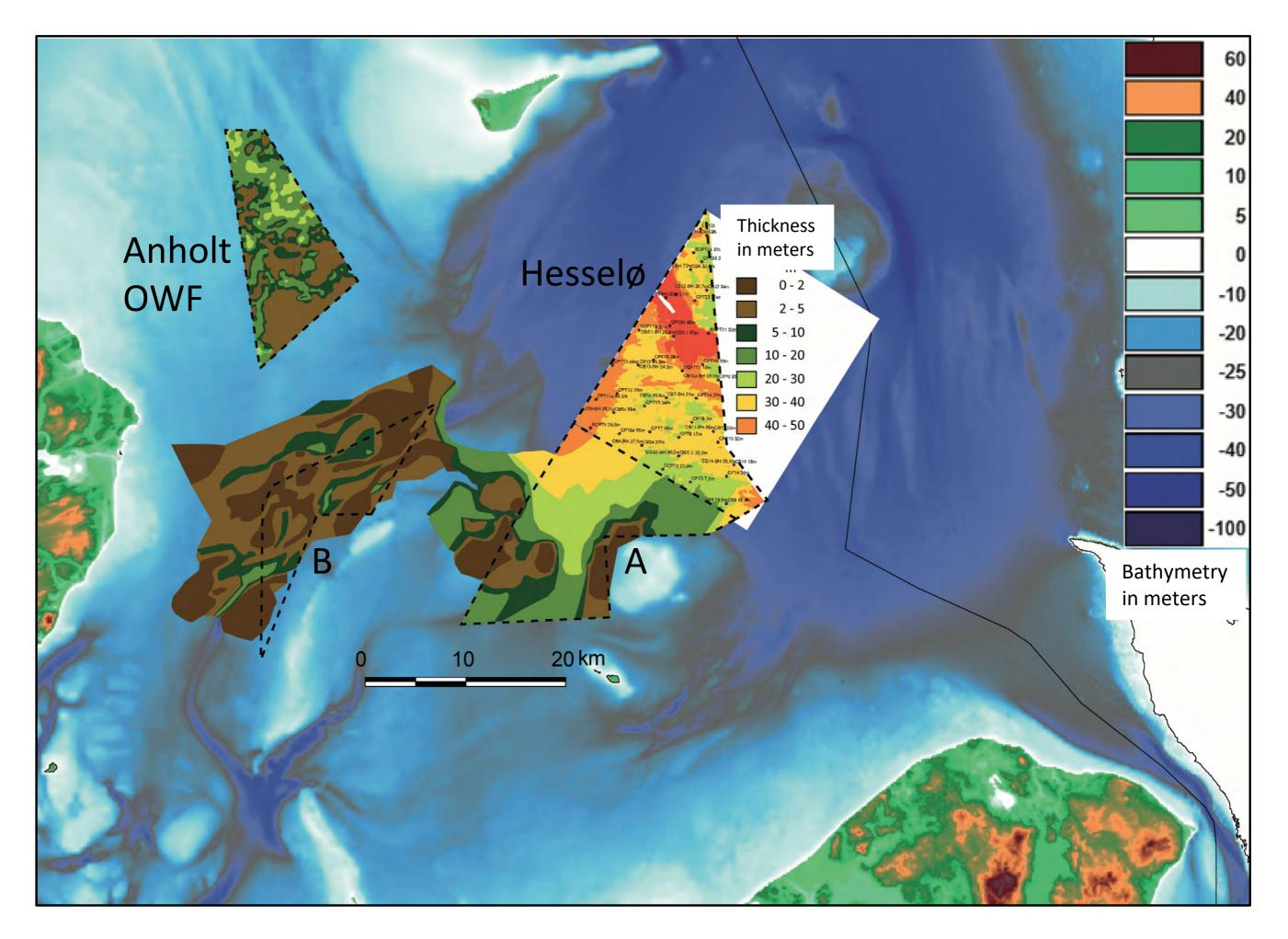
Appendix C. Hesselø, area A, B and Anholt Windfarm soft sediment thickness
