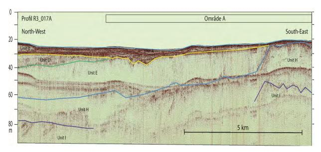
Figure 9.3 North-west to south-east section from the northern part of Area A. For details see Appendix B. Location see Figure 9.1. The seismostratigraphic units are presented in Table 1.
