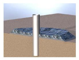
Figure 16. Example of scour protection
