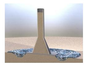
Figure 17. Example of scour protection
