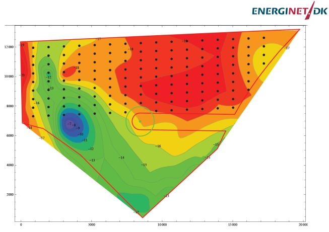
Figure 8. Suggested layout for the 3.0MW turbine at Horns Rev 3, located in the centre of the area.
