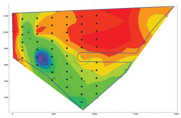
Figure 12. Suggested layout for the 8.0MW wind turbine at Horns Rev 3, located most westerly in the area.
