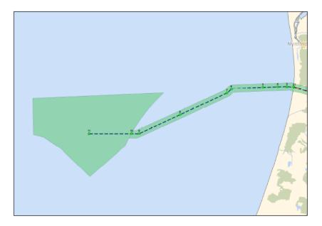
Figure 1. Location of the Horns Rev 3 OWF (400 MW) and the projected corridor for export cables towards shore. The area enclosed by the polygon is app.  $160 \text{ km}^2$ .
