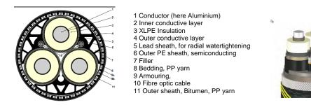
Figure 18. Illustration of a typical export cable. To the left the cross section, and the cable to the right.
