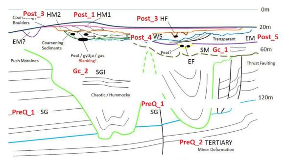
Figure 5. Horns Rev 3 Geological Model (COWI February 2014)
