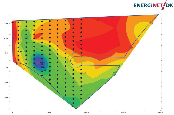
Figure 11. Suggested layout for the 3.0MW turbine at Horns Rev 3, located most westerly in the area.
