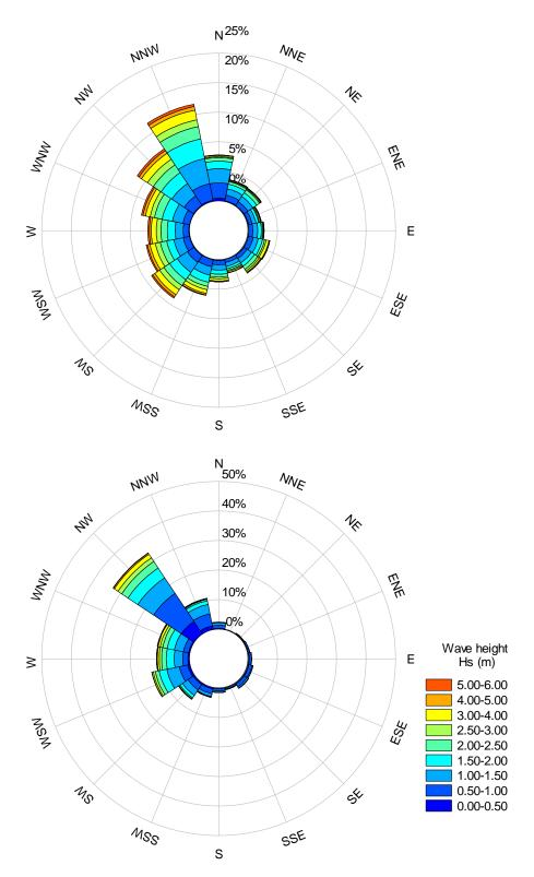
Figure 3.8. Significant wave height at the offshore Gorm platform (top) and the nearshore Nymindegab station (bottom).
