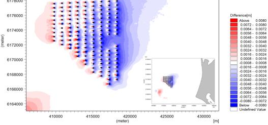
Figure 10.8. Simulated one-year return period significant wave heights (m) approaching from the west (top panel) and the change in significant wave heights (m) due to the foundation layout (bottom panel) (inset: with coast).
