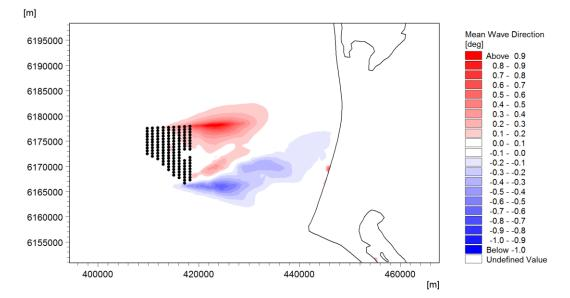
Figure 10.14. Change of wave direction by wind reduction in the lee of Horns Rev 3 (positive means wave height is increased).
