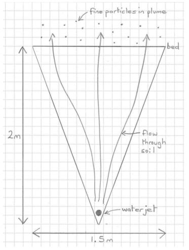
Figure 6.6. Process of jetting in cross-section.
