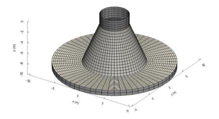
Figure 6.1. Cross-section (top) and numerical mesh (bottom) of a 3MW GBS foundation in a water depth of 10m.
