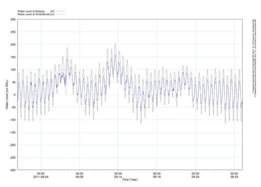
Figure 3.3. Water levels measured at Esbjerg and Hvide Sande tide gauges for September 2011.
