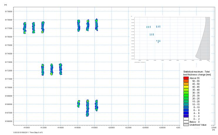
Figure 9.6. Maximum deposition (mm) from plume for the construction phase for GBS foundations and inter-array cable installation combined, including the coast (top) and zoomed in (bottom).
