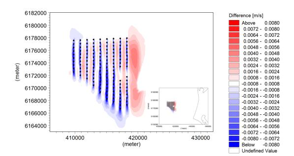
Figure 10.5. Simulated maximum tidal current velocities (m/s) (top panel) and the maximum change in tidal current velocities (m/s) due to the foundation layout (bottom panel).
