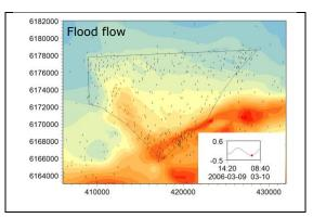
Figure 7.9. Simulated tidal currents for the baseline condition for a neap tide.
