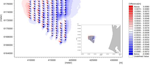
Figure 10.7. Simulated 50-year return period significant wave heights (m) approaching from the northwest (top panel) and the change in significant wave heights (m) due to the foundation layout (bottom panel) (inset: with coast).
