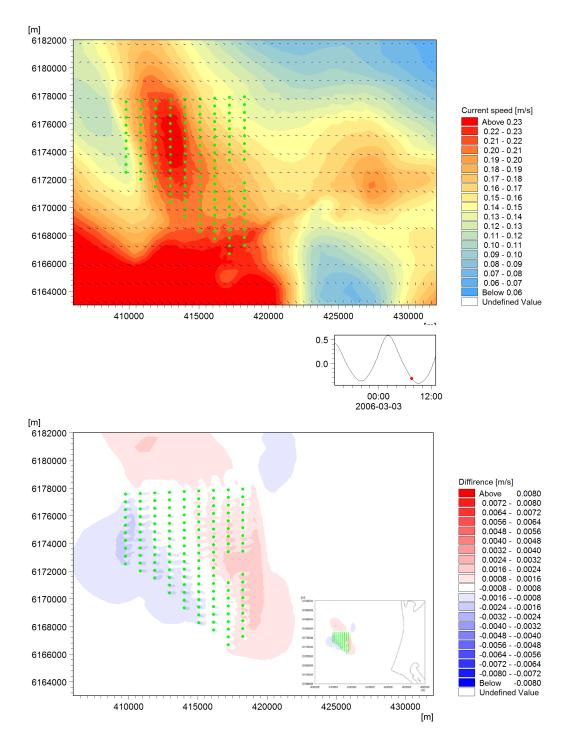
Figure 10.3. Simulated tidal current velocities (m/s) during a slack spring tide (top panel) and the change in tidal current velocities (m/s) due to the foundation layout (bottom panel).
