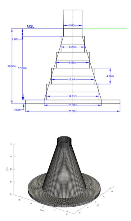
Figure 6.3. Cross-section (top) and numerical mesh (bottom) of a 3MW GBS foundation in a water depth of 20m.
