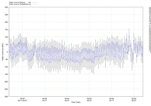
Figure 3.2. Water levels measured at Esbjerg and Hvide Sande tide gauges for April and May 2011.
