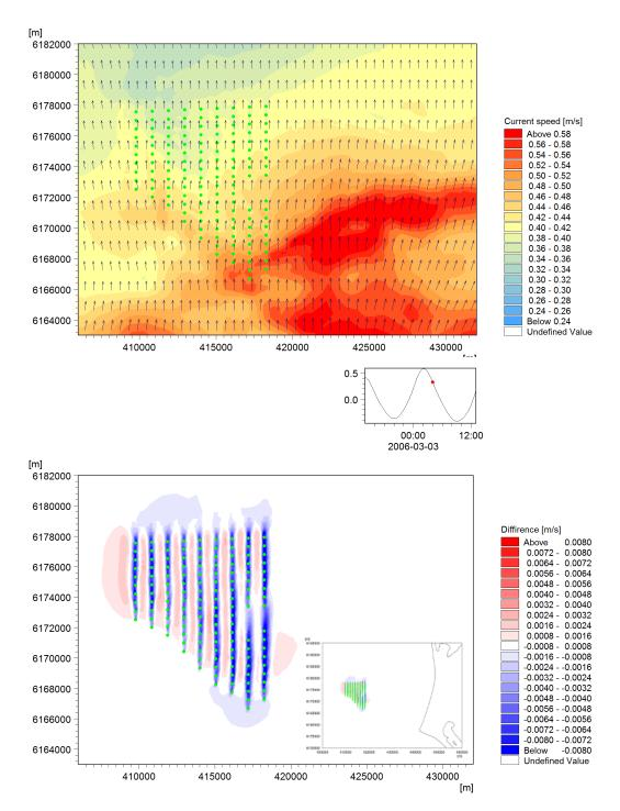
Figure 10.1. Simulated tidal current velocities (m/s) during a spring ebb tide (top panel) and the change in tidal current velocities (m/s) due to the foundation layout (bottom panel).
