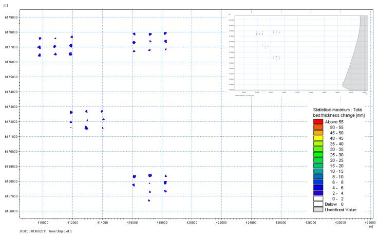
Figure 9.5. Deposition (mm) from plume for the construction phase for GBS foundations, including the coast (top) and zoomed in (bottom).
