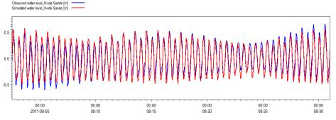
Figure 7.5. Time series comparison between simulated (red) and recorded (blue) tidal levels at Hvide Sande.
