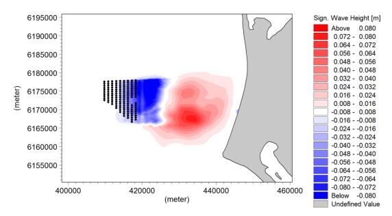
Figure 10.13. Change of wave height by wind speed reduction in the lee of Horns Rev 3 (positive means wave height is increased).
