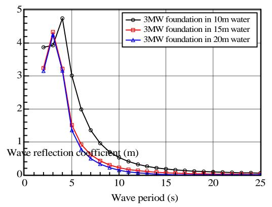
Figure 6.4. Wave reflection coefficients of 3MW GBS foundations in 10m, 15m and 20m water depth.
