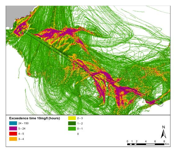
Figure 7-7 Exceedance time of suspended sediments along the cable corridor during the modelled construction phase of 27 days.
