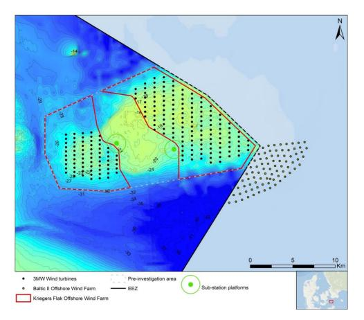
Figure 3-2 Layout of 203 wind turbines on Kriegers Flak using 3 MW turbines only.
