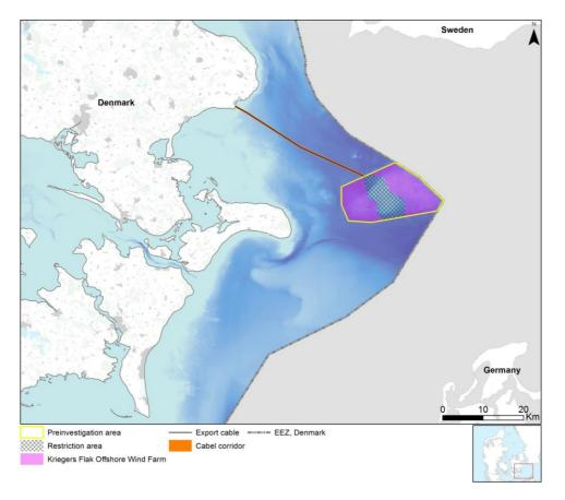
Figure 3-1 The planned location of Kriegers Flak Offshore Wind Farm (600 MW) in the Danish territory. Approximately in the middle of the pre-investigation area an area (ca. 28 km<sup>2</sup>) is reserved for sand extraction with no permission for technical OWF components to be installed (hatched area). The cable corridor shown on the figure contains two export cables. The final positions of the cables within the cable corridor have not yet been determined.
