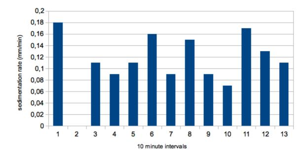
Figure 7-3 Time series of sedimentation rate during installation of a representative single 3 MW wind turbine (gravity based foundation) on Kriegers Flak OWF. Each bar represents the maximum sedimentation rate (in mm/min) observed in the 50x50 m model cells with sedimentation (NIRAS 2014).
