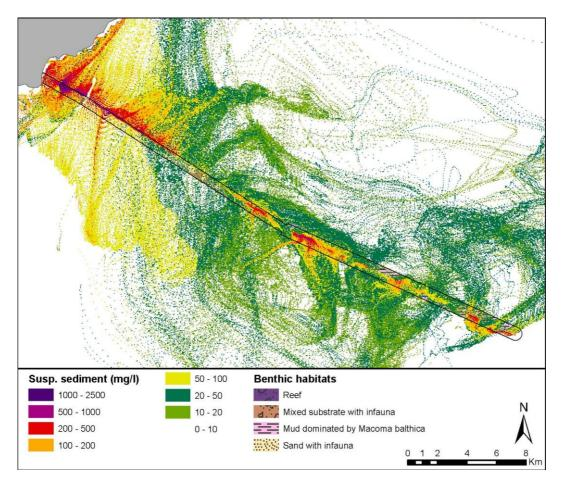
Figure 7-6 Maximum concentration of suspended sediments along the cable corridor during the modelled construction phase of 27 days.
