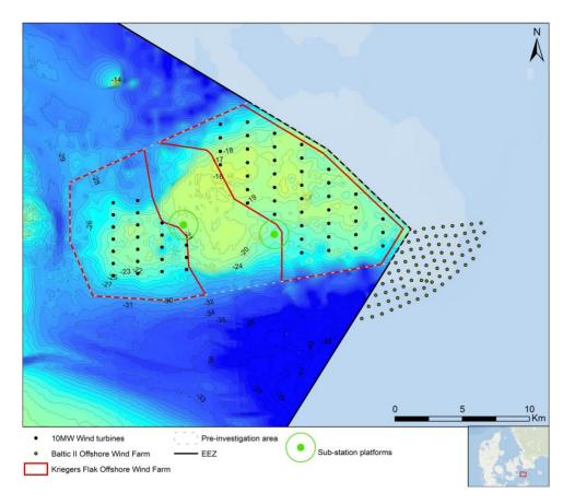
Figure 3-3 Layout of 64 wind turbines on Kriegers Flak using 10 MW turbines only.
