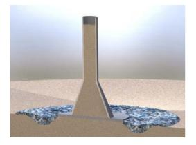
Figure 3-5 Example on scour protection for a concrete gravity base (drawing: Rambøll).
