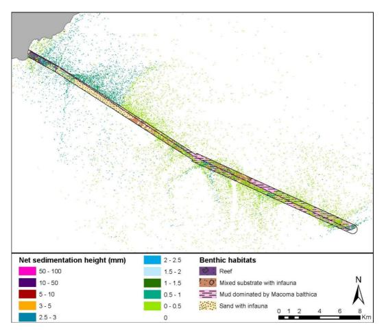
Figure 7-8 Net sedimentation at the end of the modelled construction phase (27 days) along the cable corridor.
