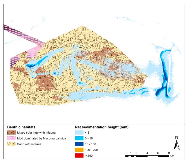
Figure 7-2 Net sedimentation thickness at the end of the construction phase. Maximum value found in the area = 1840 mm in one single model cell, otherwise maximum of 180 mm (NIRAS 2014). This scenario reflects the installation of 3 MW turbines on gravity foundations, the substations and the inter-array cables.
