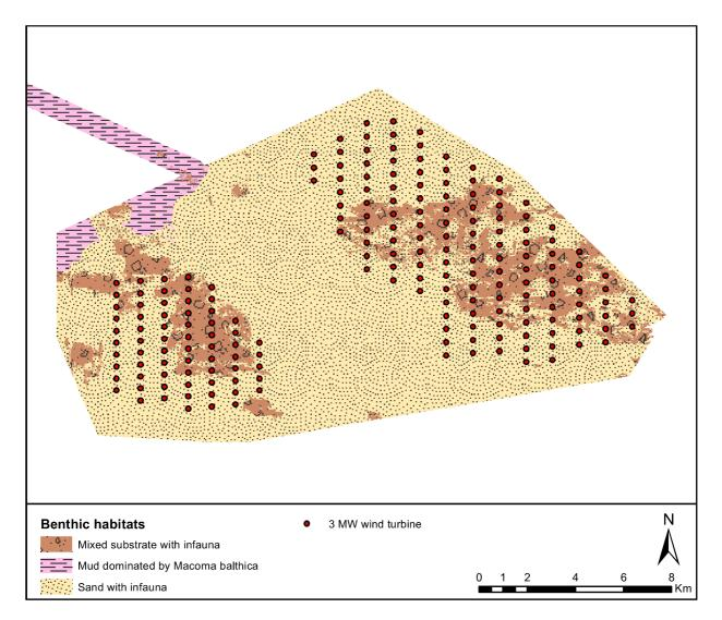
Figure 7-5 Placement example of 3 MW wind turbines on Kriegers Flak used in the impact assessment.
