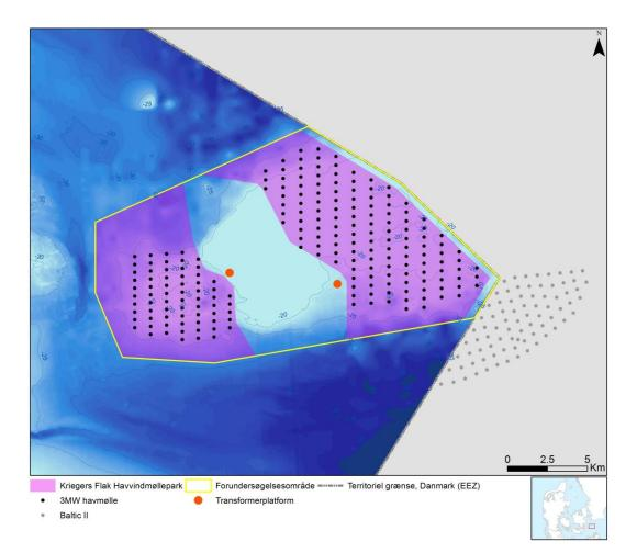
Figure 3: Suggested layout for 3.0 MW turbines at the eastern and western part of the planned wind farm (purple polygons) at Kriegers Flak at Danish territory. The two red spots indicate the position of the offshore sub-station platforms. The yellow line delineates the pre-investigation area. In the south-eastern part of the map turbines within the German Baltic II OWF are shown.
