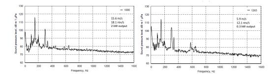
Figure 12: Measurements of noise from turbine in Horns Reef Offshore Wind Farm running close to maximum power rating (left) and at low level (right). Turbine noise consists of multiple peaks at discrete frequencies, which rise above the background noise. From: Betke (2006).
