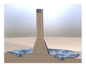
*Figure 6: Example on scour protection of a concrete gravity base (drawing: Rambøll).*
