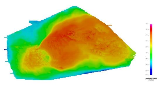
*Figure 2: Overview of the Kriegers Flak area showing water depth variations by graded colour (based on the geophysical survey).*
