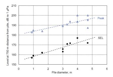
Figure 10: Measured peak levels and broadband SELs at 750 m versus pile diameter from various pile driving operations. Compiled by Matuschek & Betke (2009).
