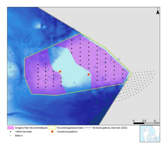
Figure 4: Suggested layout for 10.0 MW turbines at the eastern and western part of the planned wind farm (purple polygons) at Kriegers Flak at Danish territory. The two red spots indicate the position of the offshore substation platforms. The yellow line delineates the pre-investigation area. In the south-eastern part of the map turbines within the German Baltic II OWF are shown.
