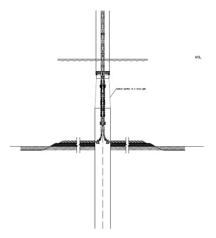
*Figure 5: The conical part of a monopile.*
