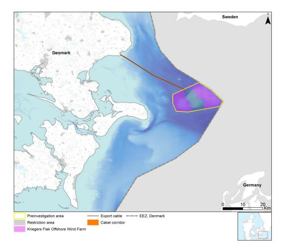
Figure 1: The planned location of Kriegers Flak Offshore Wind Farm (600 MW) in the Danish territory. Approximately in the middle of the preinvestigation area an area (c. 28 km<sup>2</sup>) is reserved for sand extraction with no permission for technical OWF components to be installed.
