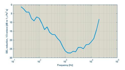
*Figure 85: Frequency dependent reduction in SEL from a bubble curtain. From Pehlke, et al., (2013).*
