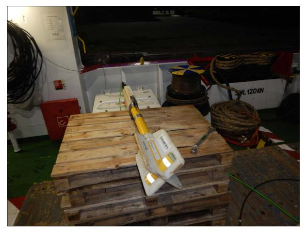
Figure 8.4: Magnetometer Spanner Test
