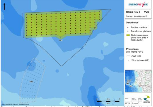
Figure 4.5Disturbance zone during operation of the OWF Horns Rev 3 (scenario with 3 MW turbines in<br/>centred position within the project area) with 500 m buffer zone around.
