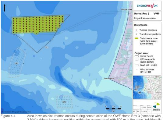
3 MW turbines in centred position within the project area) with 500 m buffer zone. Additionally locally disturbances will occur along the cable trays during installation of the Horns Rev 3 subsea cable.
