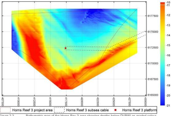
Figure 2.2 Bathymetric map of the Horns Rev 3 area showing depths below DVR90 as graded colour. The map is based upon the Geophysical survey in 2012.
