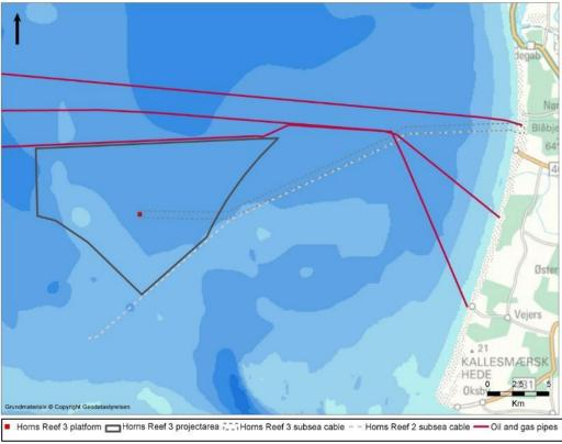
Figure 2.1 Location of the Horns Rev 3 OWF (400 MW) and the projected corridor for export cables towards shore. The area enclosed by the polygon is app. 150 km<sup>2</sup>. The marked area includes the whole pre-investigation area, i.e. with an overlap of existing cables etc.
